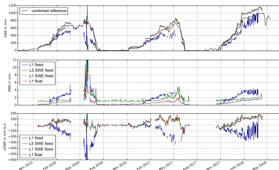
Figure 6. GPS based SWE estimation (top) and its RMS (middle) from different ambiguity resolution strategies. The black line shows the mean SWE of the three reference sensors. The bottom plot shows the differences of GPS based SWE estimation from different ambiguity resolution strategies to the mean SWE of the three reference sensors.
