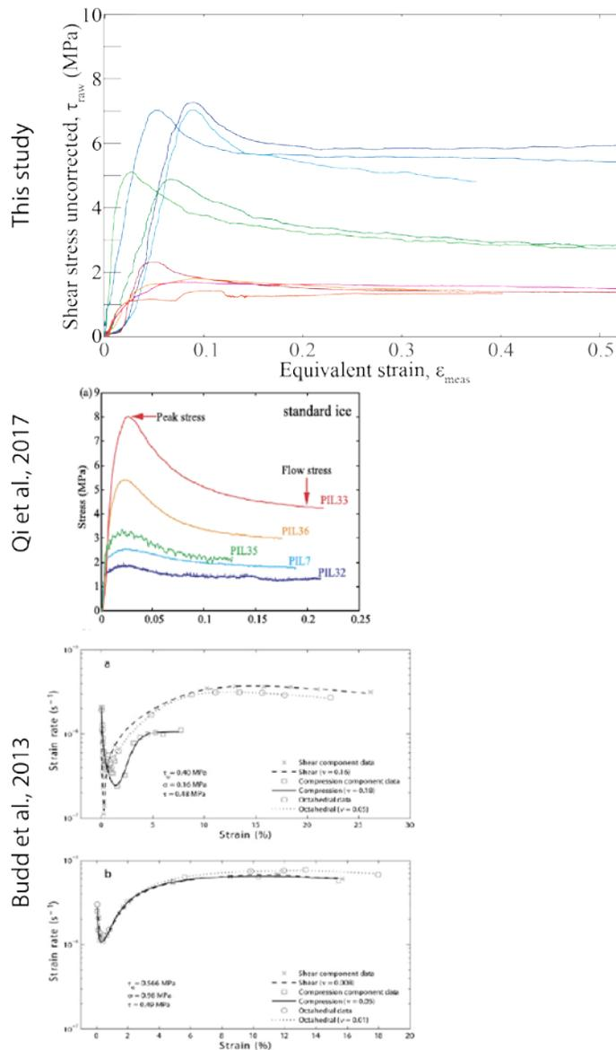
Figure 1. Plots of stress/strain rate vs. strain. All strains are equivalent to axial compressive strains.
