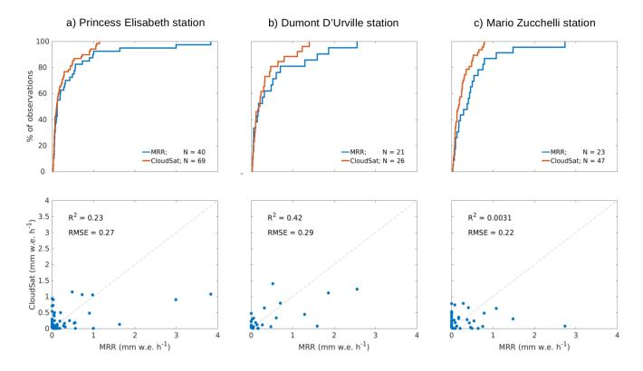
**Figure 7.** (first row) Empirical cumulative distribution of MRR and CloudSat snowfall events at a spatial resolution of  $1^{\circ}$  latitude by  $2^{\circ}$  longitude. (second row) Direct comparison between MRR and CloudSat individual snowfall events. R<sup>2</sup> denotes the adjusted coefficient of determination, RMSE is the root mean square error, while the thin line is the bisector.
