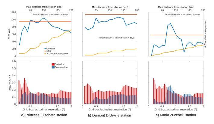
Figure 6. (first row) Overview of the total snowfall amounts for the three stations as observed by CloudSat and the Micro Rain Radars during the periods of collocated measurements (Fig. 2). (second row) Individual snowfall event error analysis. MRR snowfall rates are considered truth. The x-axis denotes different spatial resolutions of the CloudSat climatology (grid box longitudinal resolution = 2 \* grid box latitudinal resolution).
