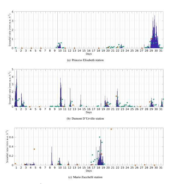
**Figure 3.** Snowfall rates (mm w.e.  $h^{-1}$ ) during March 2016 at the three stations derived from the MRRs (blue bars), the grid box comprising each of the three stations in ERA-Interim reanalysis (green) and the average of the CloudSat overpasses in the grid box (1° latitude by 2° longitude) comprising each of the three stations following the approach of Palerme et al. (2014) (red).
