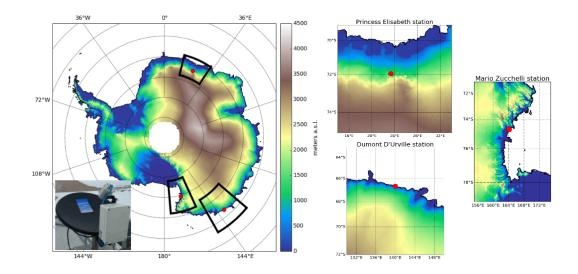
Figure 1. Digital Elevation Map of the Antarctic Ice Sheet (Liu et al., 2015) with three insets corresponding to the location of the Micro Rain Radars. Upper: Princess Elisabeth station, right: Mario Zucchelli station, lower: Dumont D'Urville station. The inset at the bottom left shows the Micro Rain Radar at the Princess Elisabeth station.
