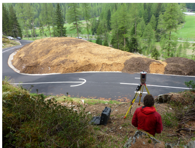
Figure 2. Martell snow heap covered with sawdust and wood chips in spring 2015. The Riegl VZ6000 laser scanner can be seen in the foreground.
