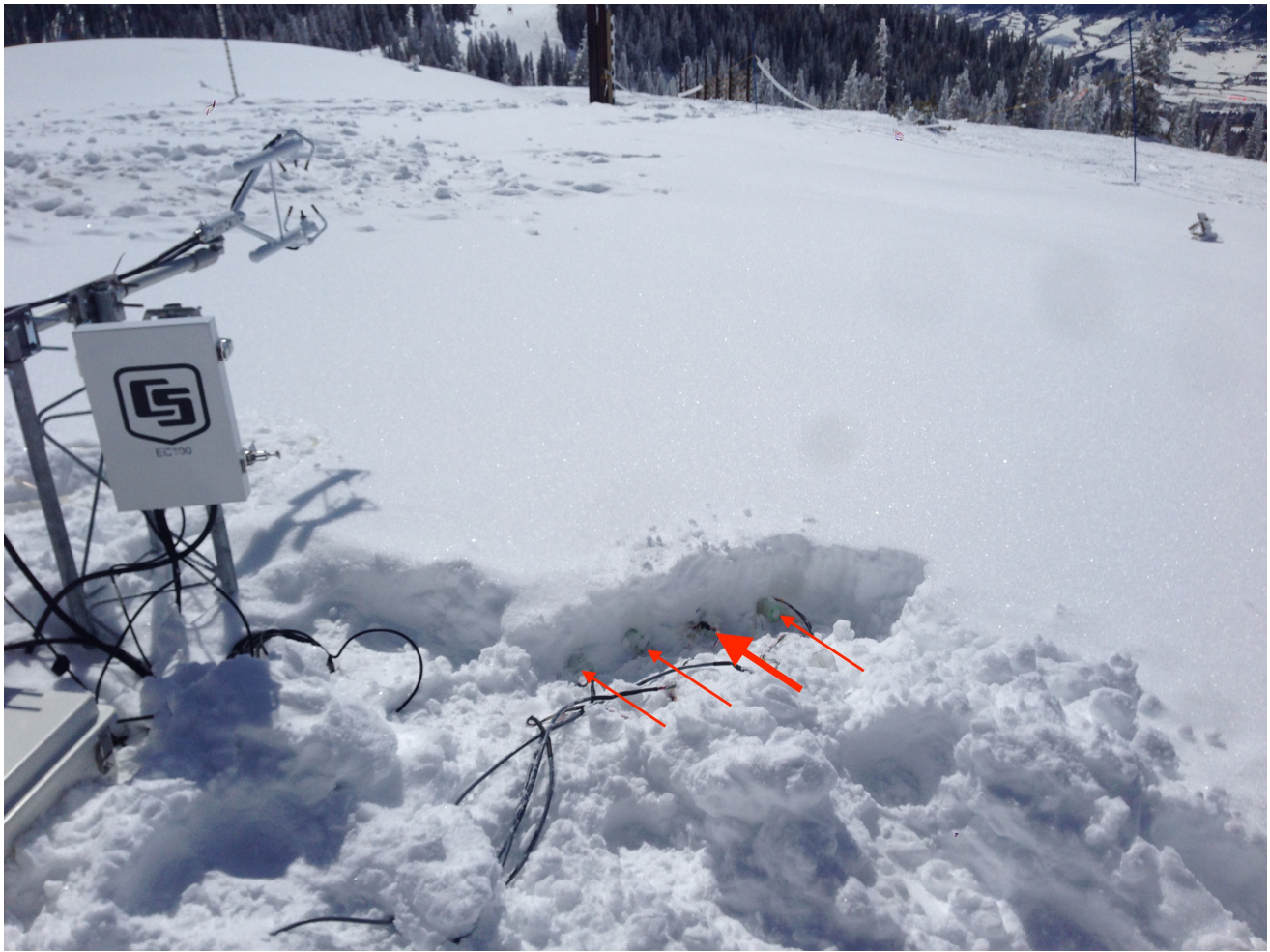
Figure 5. This picture shows the experimental setup for cases 13 and 14 and was taken after the data acquisition period. Red arrows point to the tops of the snow pickets after we removed snow to expose the top and left side of the instrumented snow layer for documentation purposes. The bold red arrow points to the snow picket where the trace gas was released for these two cases. A Campbell Scientific Irgason mounted above the snow pickets acquired horizontal and vertical wind speed and direction at 20 Hz.
