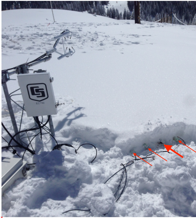
Figure 5. This picture shows the experimental setup for cases 13 and 14 and was taken after the data acquisition period. Red arrows point to the tops of the snow pickets after we removed snow to expose the top and left side of the instrumented snow layer for documentation purposes. The bold red arrow points to the snow picket where the trace gas was released for these two cases. A Campbell Scientific Irgason mounted above the snow pickets acquired horizontal and vertical wind speed and direction at 20 Hz.
