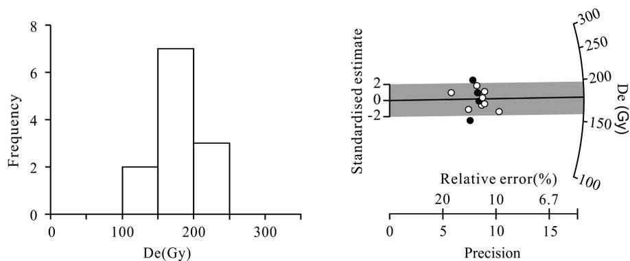
Figure 3:  $D_e$  distribution histogram (left) and radial plot (right) showing the distribution of  $D_e$  results for the fine grains. The shaded region represents  $2\sigma$  width of the distribution. The filled symbol represents the aliquots that were excluded in the final age calculation.
