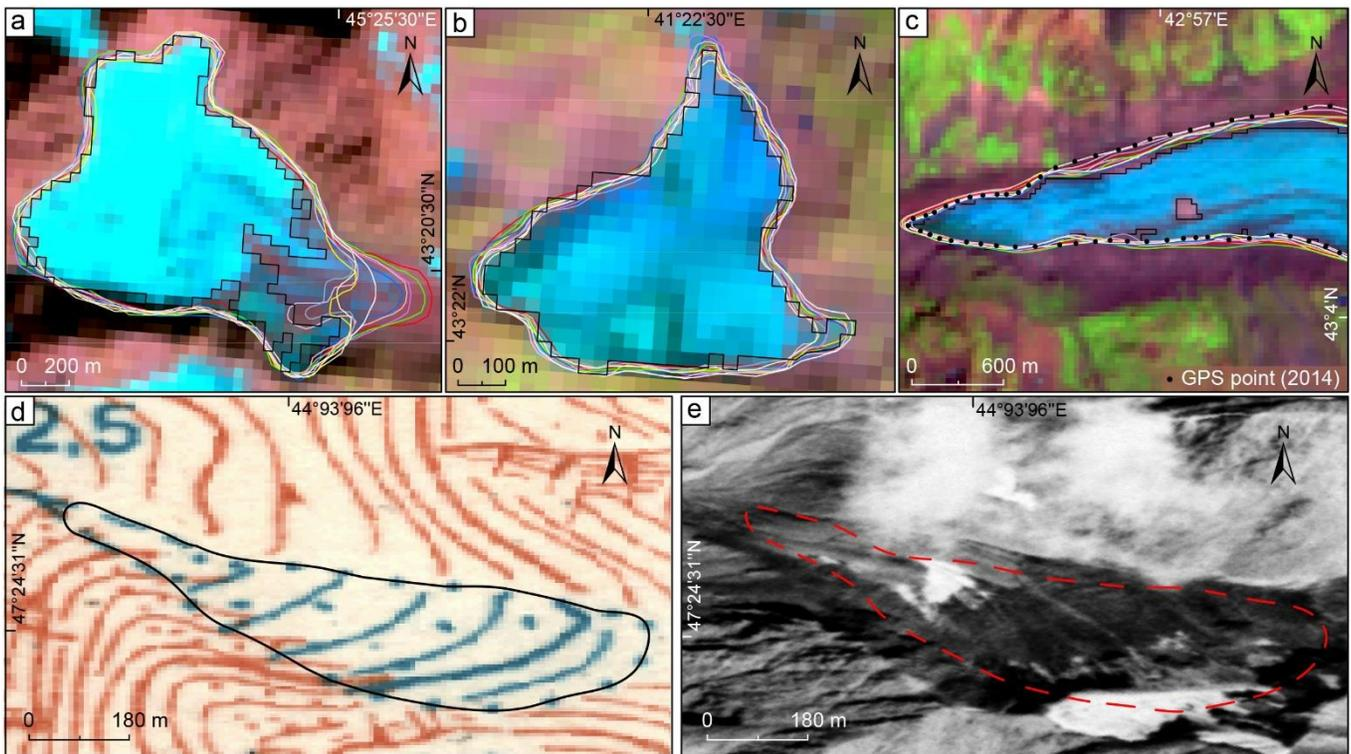
**Figure 2.** a-c Examples from the multiple digitizations of glaciers (bands 654 as RGB) using the OLI scene performed by different analysts (coloured lines). Black outlines refer to the automatically derived extents (4/6 ratio); pixel size is 30 m. d – Error in the 1960 map included mapped snow for small cirque type glacier; e – same place 1964 Corona imagery.
