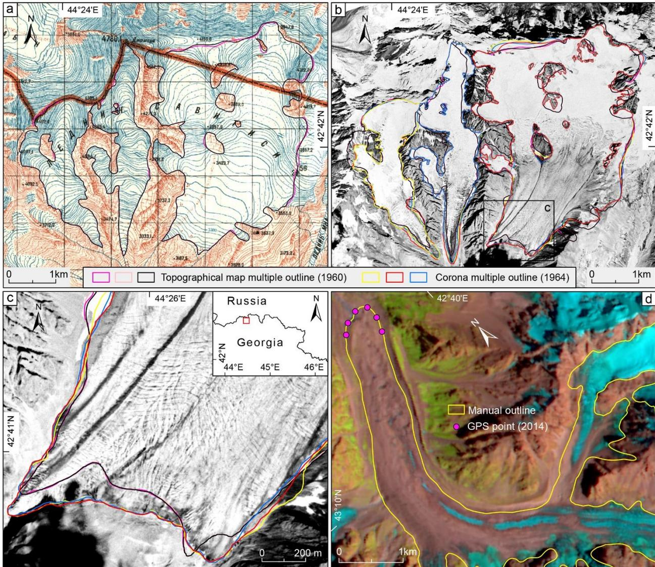
**Figure 3.** a-c Examples from the multiple digitizations of glaciers using the 1960s topographic map and 1964 Corona imagery performed by different analysts (coloured lines). d – Shkhelda Glacier, one of the heavily debris covered glaciers in the Greater Caucasus. The 23/08/2014 Landsat 8 image (Table 1) is used as background.
