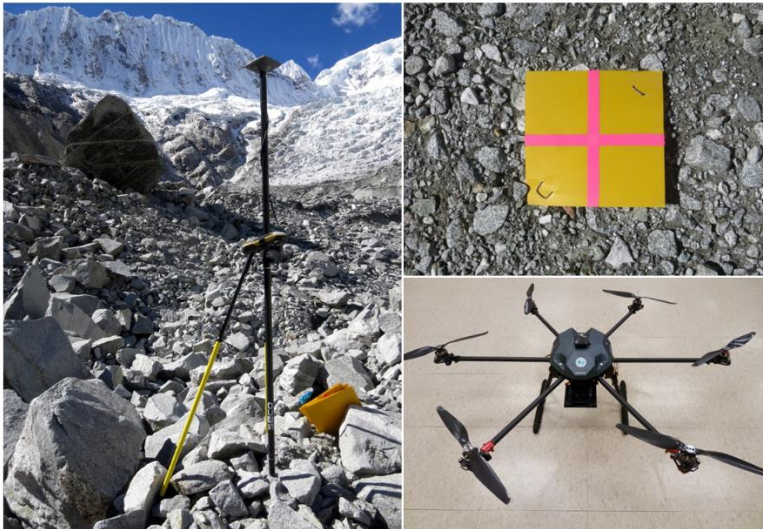
Figure 2: GNSS survey at Llaca glacier (left), installed ground control target (2015) (top right), hexacopter UAV platform used in this study (bottom right).
