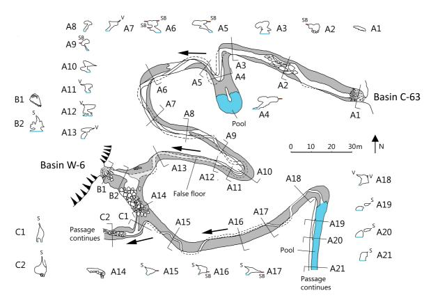
Fig. 4: Plan and passage cross sections, englacial conduit NG-04. SB: sediment band, S: 918 suture, V: voids. Standing water on the cave floor is shown in blue. For location, see Fig. 2e. 919
