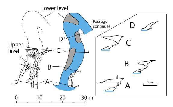
Fig. 6: Plan and passage cross sections, conduit NG-05. For location see Figure 2a.
