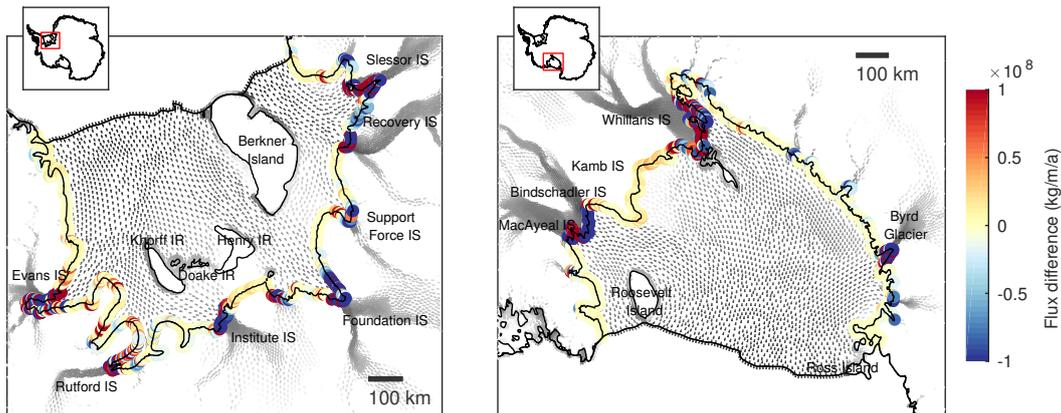
**Figure 5.** Difference between the analytical and the modeled fluxes along the grounding lines of Filchner-Ronne Ice Shelf (left panel) and Ross Ice Shelf (right panel). Analytical fluxes are calculated based on  $\theta_1$  defined in Eq. 11. In locations where the formula yields unphysical results, fluxes are set to zero. Grey arrows show the modeled ice flow. IS denotes ice streams, IR denotes ice rises or rumpled. Grounding line and ice front locations are indicated in black.
