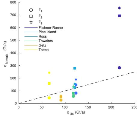
**Figure B4.** Comparison of fluxes calculated with  $\dot{U}_a$  ( $x$ -axis) and with the extended flux formula ( $y$ -axis), integrated along the grounding lines of exemplary the ice shelves indicated in the legend. Symbols indicate the different definitions of  $\theta$  as described in Sect. 3. All other parameters agree with the reference run (indicated by a circle). The dotted-dashed line shows where fluxes calculated with  $\dot{U}_a$  and predicted by the formula would agree.
