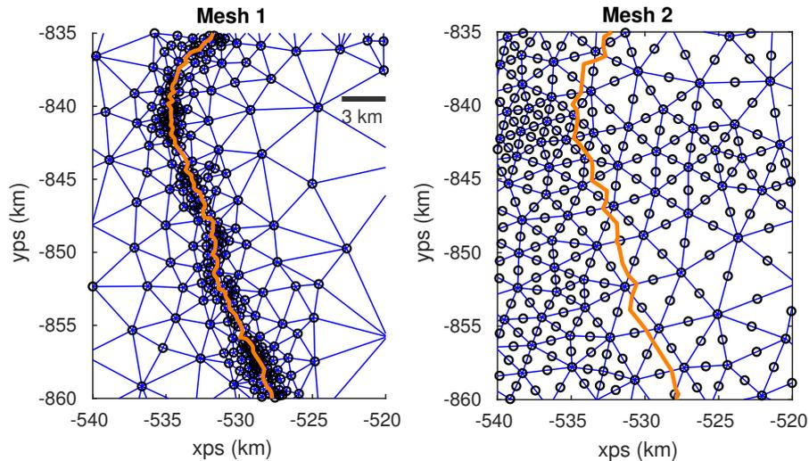
**Figure B1.** ~~Exemplary zoom~~ [Zoom](#) into the Bindschadler grounding line for two different meshes. Left panel: elements and nodes of the mesh presented in the main text. The mesh was refined especially around the grounding line and linear 3-node elements were employed. Right panel: alternative mesh with 6-node elements with quadratic base functions. The grounding line position is indicated in both meshes in orange.
