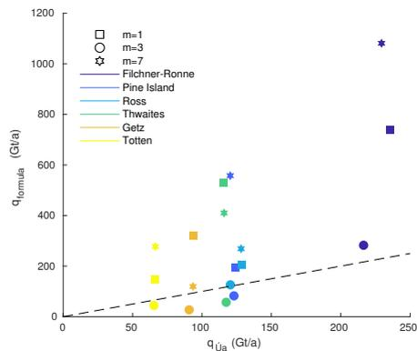
**Figure B3.** Comparison of fluxes calculated with  $\dot{U}_a$  (x-axis) and with the analytical flux formula (y-axis), integrated along the grounding lines of exemplary the ice shelves indicated in the legend. Symbols indicate the different sliding law exponents  $m = 1, 3, 7$  employed. All other parameters agree with the reference run (indicated by a circle). The dotted-dashed line shows where fluxes calculated with  $\dot{U}_a$  and predicted by the formula would agree.
