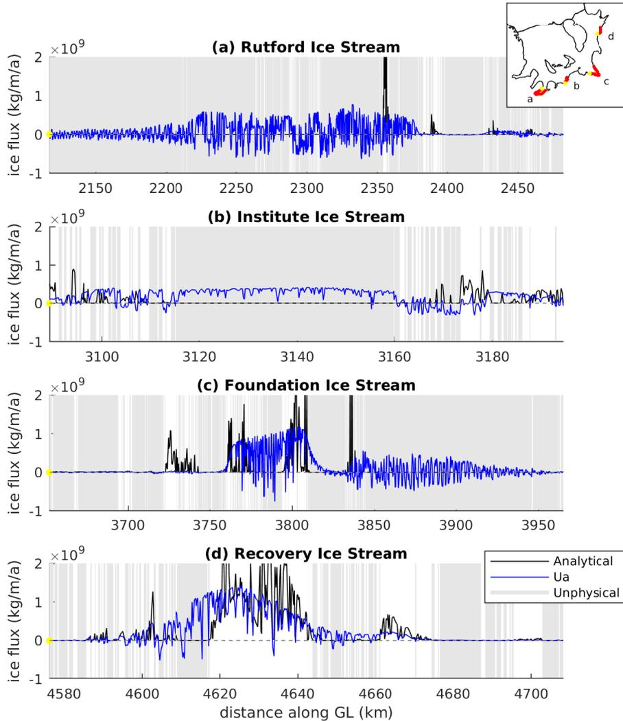
**Figure 4.** Comparison of fluxes calculated with  $\dot{U}_a$  (blue) and analytical fluxes (black) along the grounding lines of four major ice streams draining into Filchner-Ronne Ice Shelf. Locations where the flux formula provides unphysical results are marked in grey. Plotted grounding line segments are located as displayed in the inset with western margins indicated by a yellow dot.
