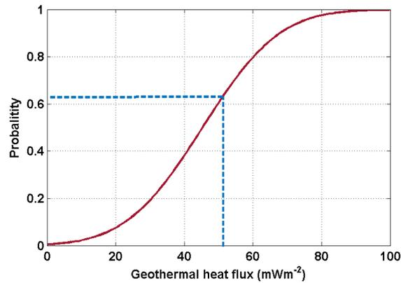
**Figure 5.** The red curve is the cumulative distribution function (CDF) based on the mean and standard deviation of Shapiro and Ritzwoller (2004) GHF data set at Dome C. The blue line is the obtained threshold  $G_{\text{pmp}}$  of  $51.6 \text{ mW m}^{-2}$ , and the indicated probability of having a GHF less than that value.
