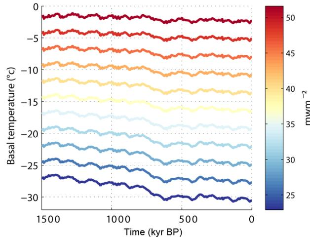
**Figure 2.** Basal temperature evolution at Dome C over a period of 1.5 Ma calculated for an ensemble of GHF values illustrated by colours. Red colours indicate high GHF values which induce temperature temperatures close to the pressure melting point, ~~on the other hand~~ blue colours show low GHF values which lead to colder basal temperatures. The GHF values on the illustration are restricted between 22 and 52  $\text{mW m}^{-2}$ .
