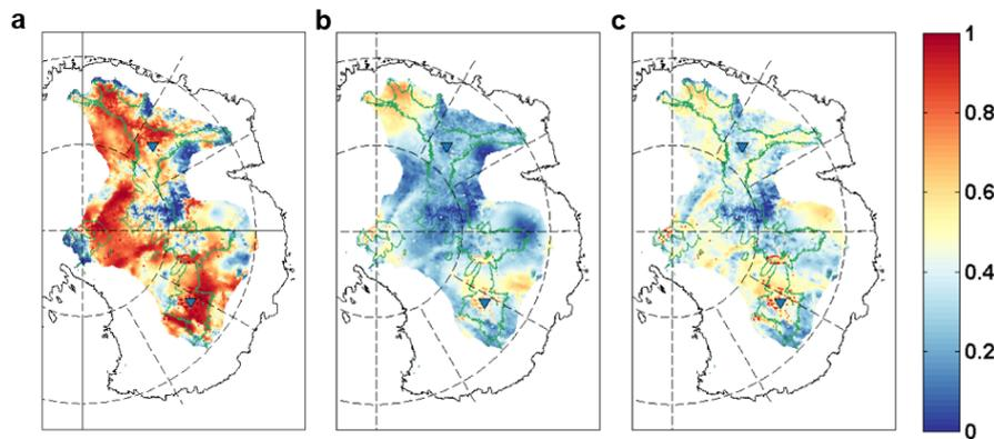
**Figure 6.** Probability that ice reached the pressure melting point over the last 1.5 Ma according to the GHF data sets from Martos et al. (2017), Purucker (2013) and Shapiro and Ritzwoller (2004), from left to right, respectively.
