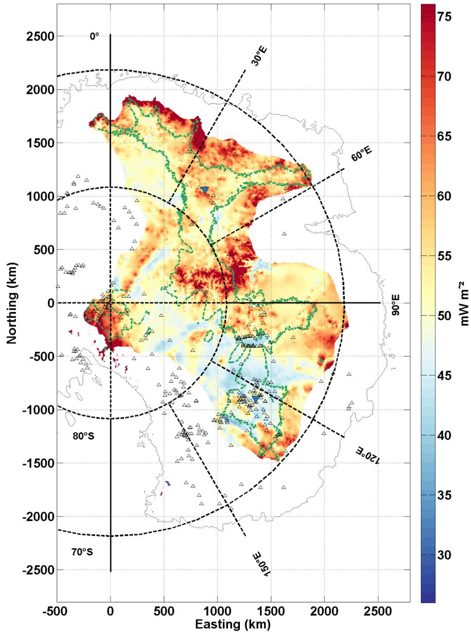
**Figure 4.** Map of  $G_{\text{pmp}}$ , i.e. the maximum GHF to keep a frozen base over 1.5 Ma. Colours represent the magnitude of the GHF ( $\text{mW m}^{-2}$ ). The colour scale's central GHF value, in yellow, is  $51 \text{ mW m}^{-2}$ . The small black triangles locate the 379 subglacial lakes (Smith et al., 2009; Wright and Siegert, 2012). [The green line outlines areas with surface velocities  \$< 2 \text{ m a}^{-1}\$  \(calculated from balance velocities, Pattyn, 2010\).](#)
