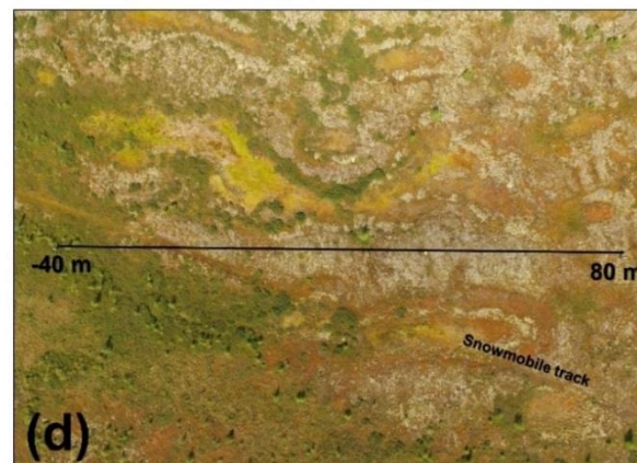
Figure 6. Peatland permafrost at Cartwright. Frost tables and modelled resistivities on (a) ERT profile 5; and (b) ERT profile 7. UAV vertical images of (c) ERT profile 5 and (d) ERT profile 7, with black lines delimiting the approximate location of the ERT survey lines and text showing the start and end points.
