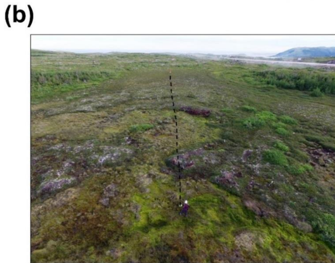
Figure 5. Peatland permafrost at Red Bay. (a) Frost tables and modelled resistivities on ERT profile 4; (b) Oblique aerial photo upslope along ERT profile 4 from the survey start point. Dotted black line delimits location of ERT survey line; (c) UAV vertical image of the site. Black line delimits the approximate location of the ERT survey line and text shows the start and end points.
