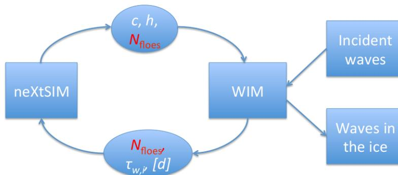
**Figure 3.** Schematic showing the information passed between neXtSIM and the WIM. Note that  $N_{\text{floes}}$  is modified by both the WIM and neXtSIM (which use different grids), so must be treated carefully to avoid numerical diffusion. Also input to the WIM are incident wave fields, and it also outputs diagnostic fields of the waves in the ice. Optional: the WIM may also update the damage  $d$ .
