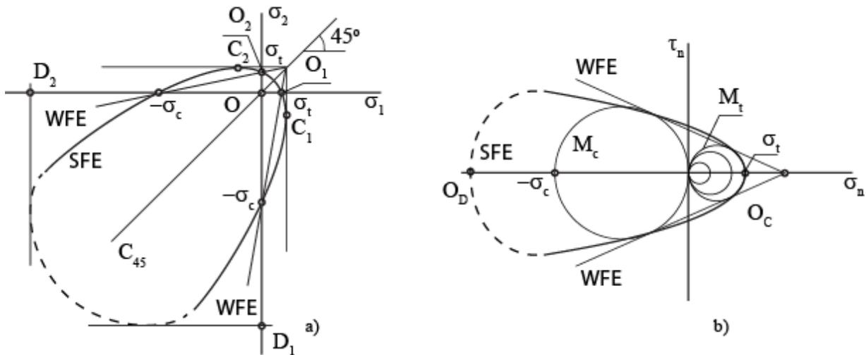
Figure 1. Ice failure envelopes on the plane of principal stresses (a) and Coulomb-Morh plane (b). SFE – Schulson’s failure envelope, WFE – Williams failure envelope.
