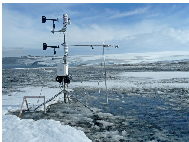
Figure 3. AWS installed on the Fourcade glacier with view to the Potter Cove and Three-Brother Hill. The photo was taken on 04 March 2012 and shows the AWS during the ablation period when pyroclastic material resurface due to melting of the winter snow layer.
