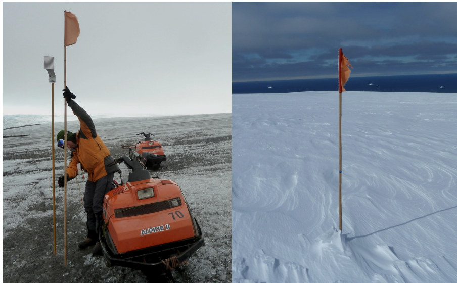
Figure 5. MBS transects installed on the Fourcade glacier during the ablation period on 28 March 2012 (left) and during the accumulation period on 10 November 2012 (right).
