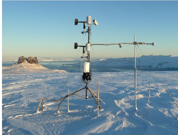
Figure 2. AWS installed on the Fourcade glacier with view to the Potter Cove and Three-Brothers Hill. The photo was taken during winter on 30 May 2012.
