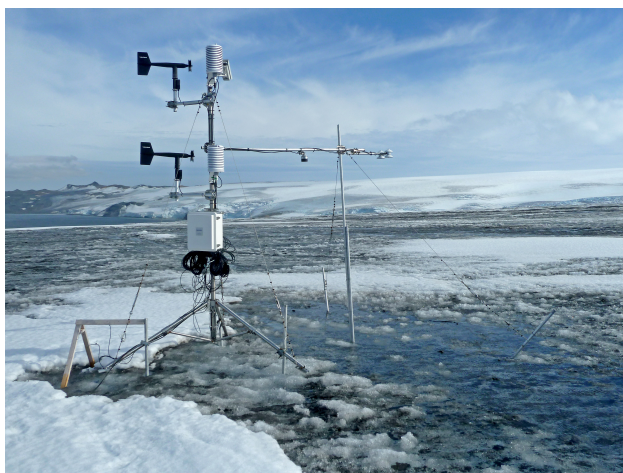
Figure 3. AWS installed on the Fourcade glacier with view to the Potter Cove and Three-Brother Three-Brothers Hill. The photo was taken on 04 March 2012 and shows the AWS during the ablation period when pyroclastic material resurface due to melting of the winter snow layer.
