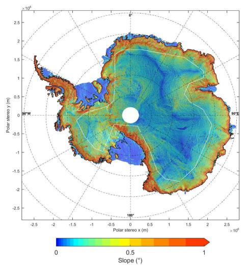
Figure 5: Surface slopes of Antarctica posted at a resolution of 1 km, derived from the digital elevation model. The mode mask boundary between CryoSat-2 LRM and SARIn modess is also shown in white.
