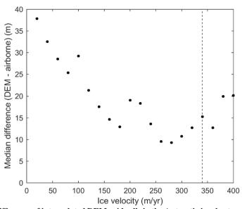
Figure AC1: Median difference of interpolated DEM grid cells in the Antarctic ice sheet evaluated against IceBridge airborne measurements, binned into ice velocity bands 20 m/yr in size. 90% of all interpolated DEM grid cells in the Antarctic ice sheet are located in regions flowing slower than 340 m/yr, shown in the vertical dashed line.
