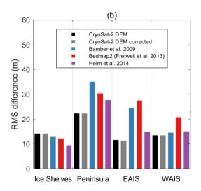
Figure 8: (a) Median and (b) RMS differences between airborne elevation measurements calculated over the ice shelves, Antarctic Peninsula, West Antarctica (WAIS) and East Antarctica (EAIS) for the new CryoSat-2 DEM presented in this report, and three publically available Antarctic DEMs. CryoSat-2 DEM comparisons with the elevation change correction applied (Table 2) are plotted as square outlines grey bars.
