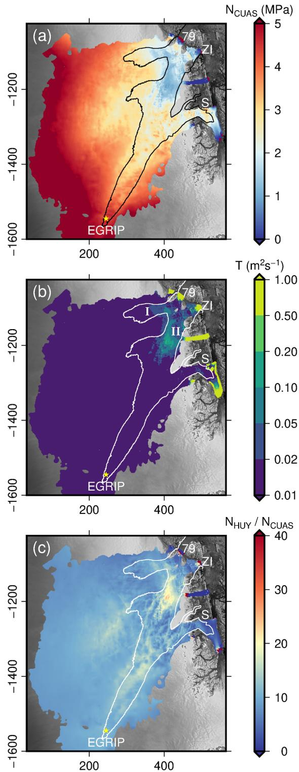
**Figure 8.** Results for NEGIS region with forcing due to basal melt (PISM) representing winter conditions. White lines indicate the  $50 \text{ m a}^{-1}$  velocity contour. Panel (a) shows effective pressure  $N_{\text{CUAS}}$ , (b) transmissivity  $T$  (logarithmic scale), and (c) shows the quotient of the ice overburden pressure above flotation and the effective pressure computed by CUAS.
