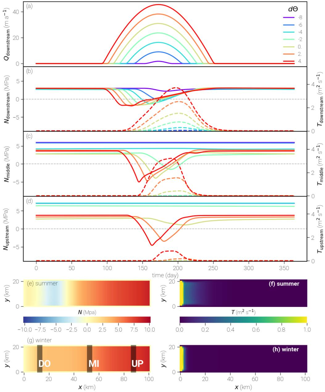
**Figure 6.** Results for one season of the SHMIP/D experiment. In panels (b)–(d), the left axis (effective pressure) corresponds to the solid lines, while the right axis (transmissivity) specifies the values for the dashed lines. The values at the given positions (upstream, middle, downstream) are averaged over the corresponding areas indicated in panel (g). Panels (e)–(h) show two-dimensional distribution maps of  $d\Theta = -4$  run.
