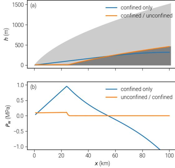
**Figure 5.** Advantages of using the confined/unconfined aquifer scheme (CUAS): Values of head and water pressure for geometries with non-flat bedrock. (a) Computed head for the confined and combined scheme with ice geometry in the background. In the confined only case, the head goes below bedrock. (b) Resulting water pressure, only for the combined scheme the pressure is always non-negative.
