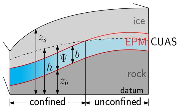
**Figure 1.** Sketch of the EPM model and artificial geometry for experiments. The left side is towards the glacier snout. Red border shows the location of the equivalent porous medium that is modelled. The blue gradient indicates the locally increased transmissivity. When  $\Psi < b$  the system becomes unconfined.
