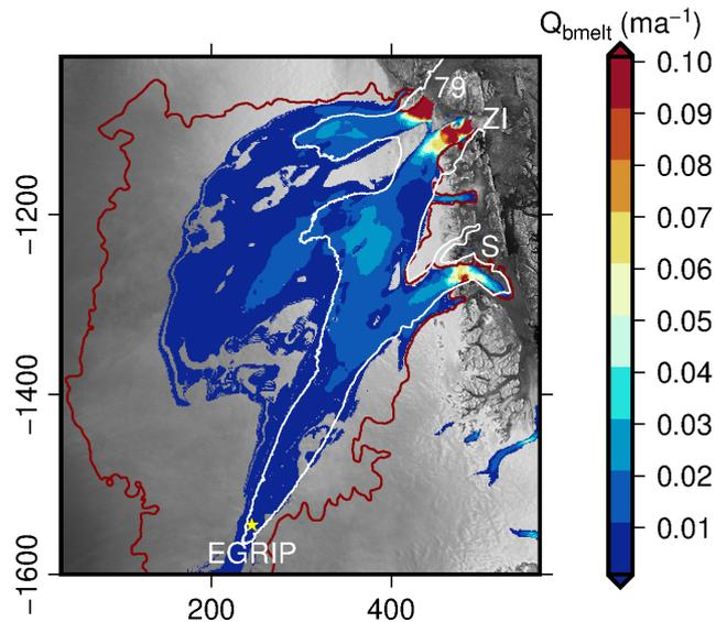
**Figure 7.** Boundary conditions and forcing for NEGIS experiment. Shown is the basal melt rate from PISM and contour line for  $\Theta_{\text{pmp}} = -0.1\text{K}$  (red) used as model boundary. The white line indicates the  $50\text{ m a}^{-1}$  velocity contour.
