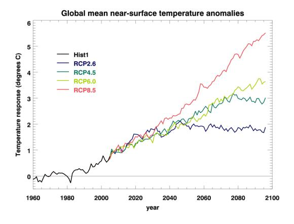
**Figure 1:** Global mean near-surface air temperature anomalies for HadGEM2ES for the IPCC CMIP5 Historical forcing scenario (black), followed by RCP8.5 (red), RCP6.0 (light green), RCP4.5 (dark green), and RCP2.6 (blue); the 1<sup>st</sup> ensemble member in each case.
