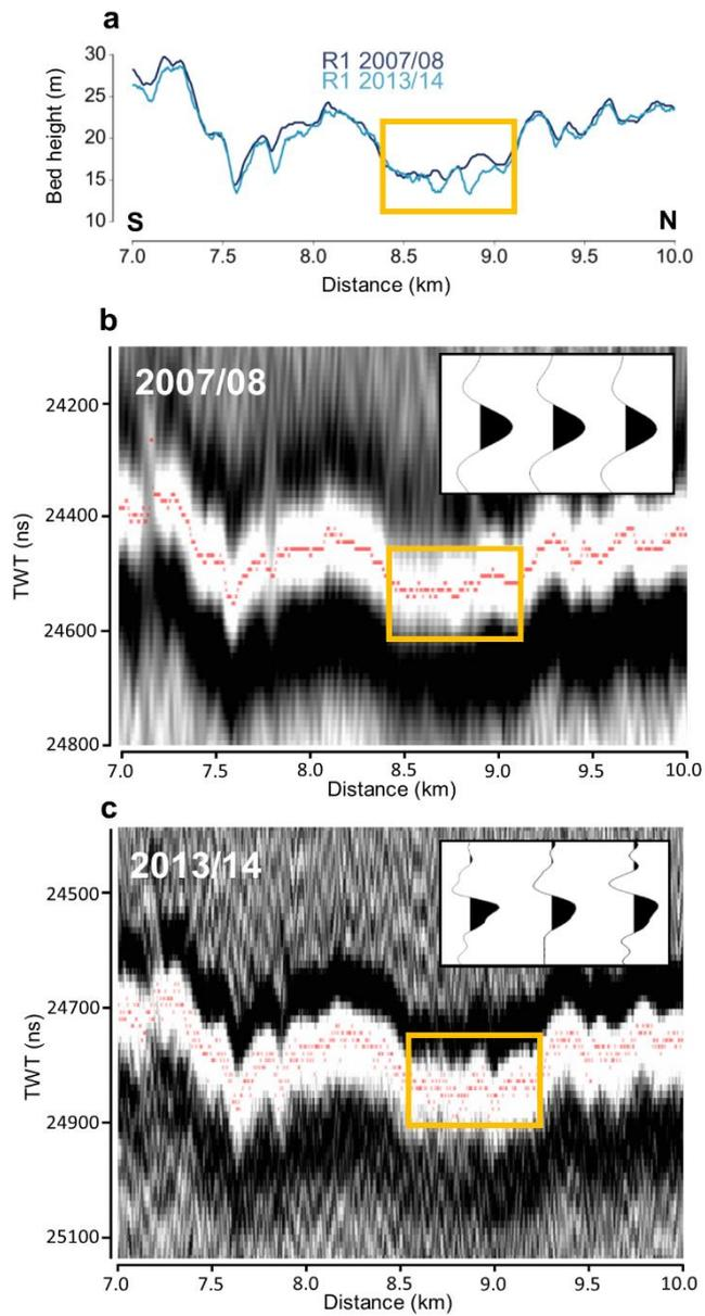
**Figure 5:** Close-up view of change in bed morphology between 2007/08 and 2013/14 identified in survey R1. Yellow boxes outline the area of change identified as having a low correlation ( $r = -0.2$ ) (a) smoothed bed picks from radar data. (b, c) raw bed picks (red dots) of the basal reflector in 2007/08 and 2013/14. Inset plots show representative traces sampled from the bed reflector.
