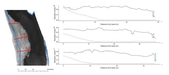
Figure 2 Cross sections through the Gaula ice jam at three different locations marked A, B and C. The height of the shear wall of the ice jam is marked with an arrow in each cross section. The dashed line indicates the ground level from the 1 meter resolution Norwegian DEM. Most
