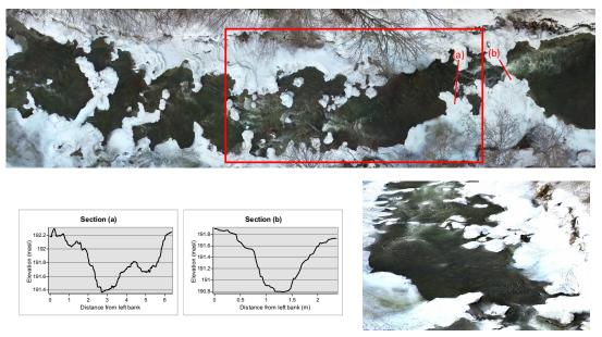
Figure 3 Partly broken anchor ice dams in the Sokna reach. The upper picture shows an orthophoto mosaic of the reach, the lower pictures shows and the two sections (a) and (b) marked on the picture and the area in the red rectangle seen from downstream.
