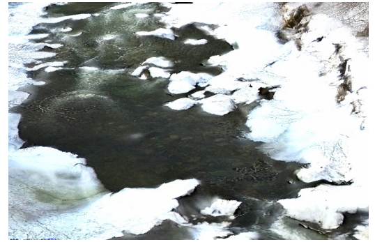
Figure 3 Partly broken anchor ice dams in the Sokna reach. The upper picture shows an orthophoto mosaic of the reach, the lower graphs shows the two sections (a) and (b) marked on the picture and the picture shows the area in the red rectangle as seen from downstream.
