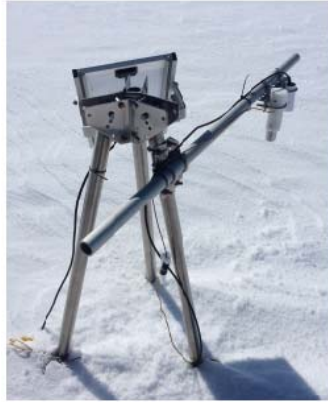
560 Figure 2: Image of the IR skin temperature sensor and tripod set up.
