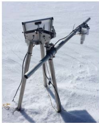
530 Figure 2: Image of the IR skin temperature sensor and tripod set up.
