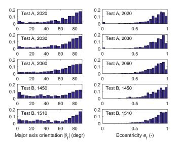
Figure 3. Histograms of the absolute value of floe orientation  $|\theta_f|$  (left) and eccentricity  $e_f$  (right) in the five analyzed tests, for floes with  $s > 5 \cdot 10^{-3} \text{m}^2$ . Bin widths equal 5° and 0.04, respectively; bar heights are normalized so that their total area in each panel equals one.
