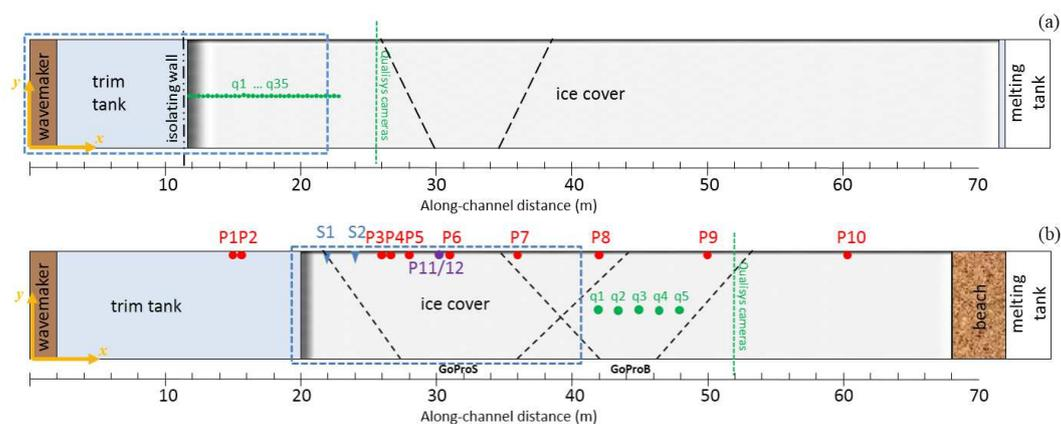
**Figure 1.** Instrument setup during Test Group A (a) and B (b): single pressure sensors are marked in red, a double pressure sensor – in violet, ultrasound sensors – in blue, Qualisys markers – in green; dashed black lines show fields of view of sideward-looking GoPro cameras, dashed blue lines – fields of view of the cameras mounted on the ceiling.
