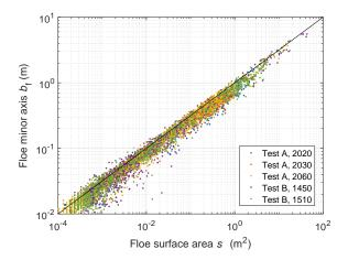
Figure 4. Scatterplot of the floe minor axis  $b_f$  (m) vs. floe surface area s (m<sup>2</sup>). Data from all five tests. The slope of the black line equals 2.
