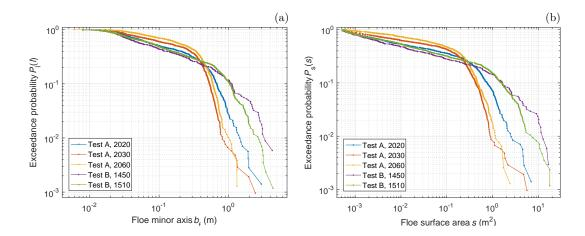
Figure 6. Log-log plots of the exceedance probability  $P_l(l)$  (a) and  $P_s(s)$  (b) for unbinned data from all five tests, for floes larger than  $5 \cdot 10^{-4}$  m<sup>2</sup>.
