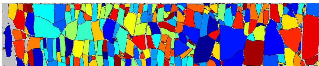
**Figure 2.** Example of a final result of the image analysis (test B, 1510), with identified ice floes marked by black contours and randomly selected colors. The ice edge is to the left, the beach to the right; the height of the image corresponds to the distance of 10 m (tank width), gray areas are open water or ice that could not be identified (very small pieces etc.). See Supplementary Figs. 2 and 3 for all analyzed images.
