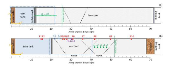
**Figure 1.** Instrument setup during Test Group A (a) and B (b): single pressure sensors are marked in red, a double pressure sensor – in violet, ultrasound sensors – in blue, Qualisys markers – in green; dashed black lines show fields of view of sideward-looking GoPro cameras, dashed blue lines – fields of view of the cameras mounted on the ceiling.
