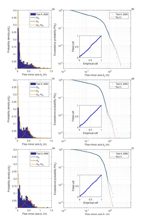
Figure 7. Results of the linear least-square fit of predicted and observed cdfs for  $b_f$  data from Test Group A: histograms of  $b_f$  with fitted  $p_{PL}$ ,  $p_G$  and  $p_l$  (a,c,e) and observed exceedance probabilities with fitted  $P_l$  (b,d,f). The insets show P–P plots of the fitted vs. observed cdfs.
