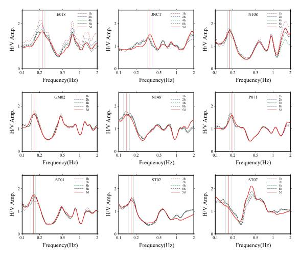
**Figure 8.** H/V spectra calculated using different lengths of ambient noise records. There is a good consistence between H/V spectra determined with different tesing length of noise records (1 h, 2 h, 4 h and 8 h) and the spectrum with record five-day long, both in locations of peak frequencies and the spectra shape. However, the peak frequency obtained from 1 h record slightly deviates the peak frequency determined using 5 d record for the E012 station.
