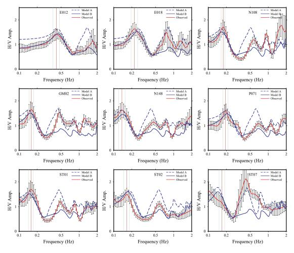
**Figure 6.** The synthetic H/V spectra and the observed H/V spectrum for the nine stations. The synthetic H/V spectra are modelled using the optimum inversion shear-wave velocity profiles for model A and model B. The two synthetic H/V spectra are both in good agreement with the observed H/V spectrum. Note that the amplitudes of the synthetic H/V spectra are normalized by dividing 2 in the whole frequency band.
