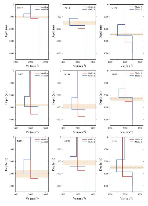
**Figure 5.** The optimum inversion shear-wave velocity models for the nine stations. The horizontal dashed line in each plot indicates the reference Bedmap2 ice thickness, and the shaded area shows the uncertainty of the Bedmap2 ice thickness. Apparently, the inversion ice thickness results derived from the two-layer structure (model B) are much closer to the Bedmap2 thickness than those determined using the single ice layer (model A).
