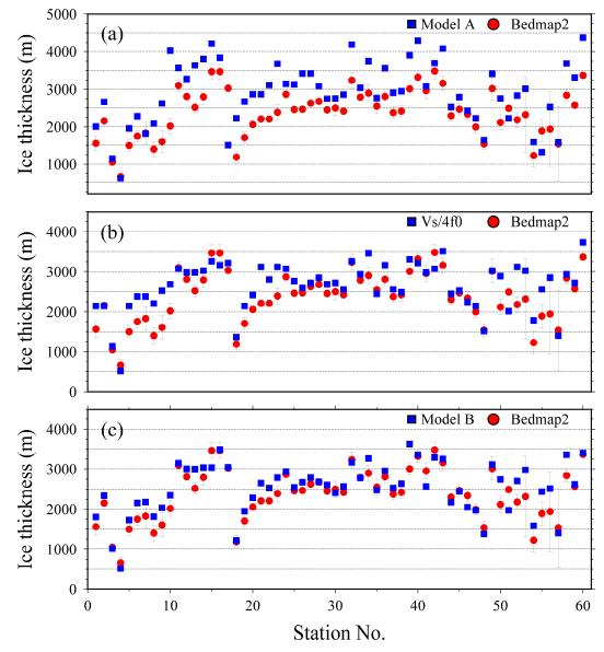
**Figure 7.** Ice thickness derived from the H/V method versus the reference Bedmap2 ice thickness. The blue squares in panel (a), (b), and (c) represent ice thickness estimations from model A, Eq. (1), and model B, respectively. The red circles in each panel denote the Bedmap2 ice thickness and each Bedmap2 value is marked with its corresponding error bar obtained from the uncertainty grids (Fretwell et al., 2013).
