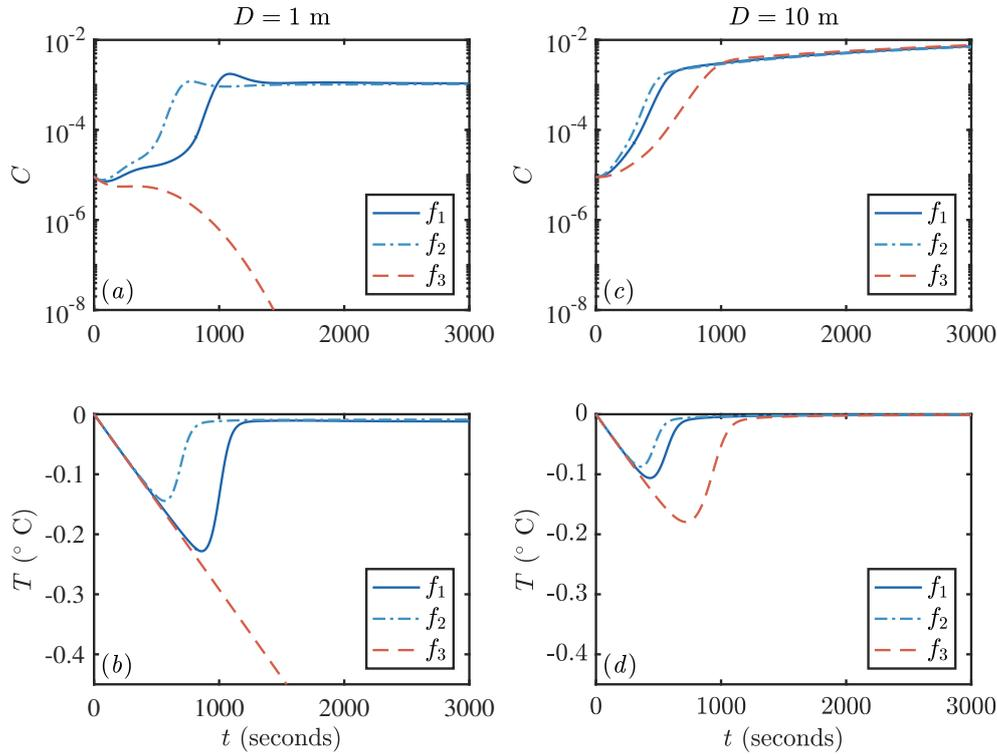
**Figure 5.** Evolution of crystal concentration (a, c), mixed-layer temperature (b, d) using the three growth rate formulae discussed in section 1.2. Using  $D = 1$  m leads to frazil explosions for growth laws 1 and 2, but the population collapses for growth law 3. For a deeper mixed layer  $D = 10$  m, all the growth laws result in a frazil explosion. Other parameters are as in Figure 2.
