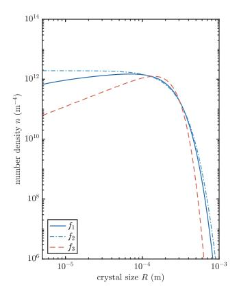
Figure 7. Numerically calculated steady-state crystal size distributions using the three growth rate formulae discussed in section 1.2. The parameters are as in Figure 2.
