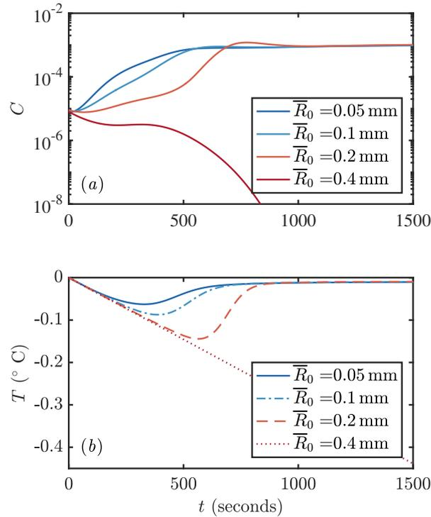
**Figure 6.** Evolution of (a) crystal concentration and (b) mixed-layer temperature using four different initial average crystal sizes (0.05, 0.1, 0.2 and 0.4 mm), growth law  $f_2$  and other parameters as in Figure 2.
