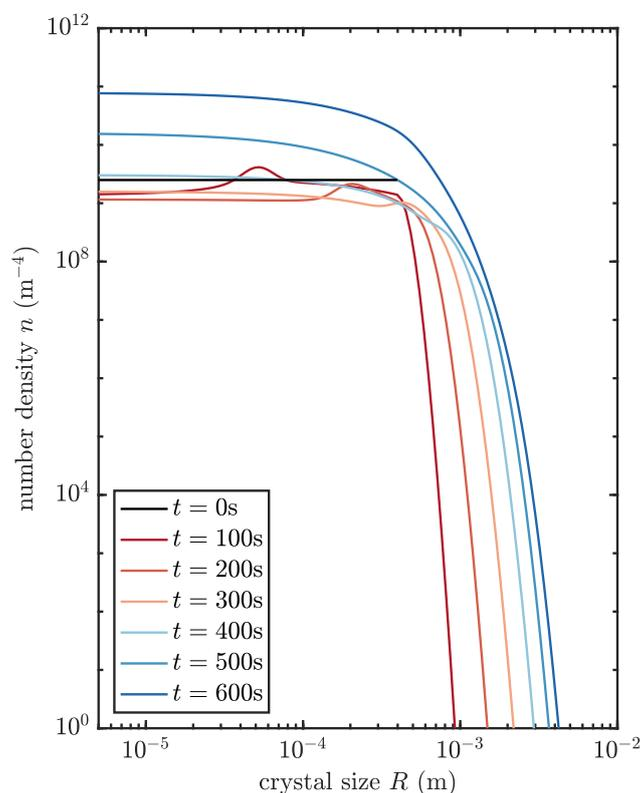
**Figure 4.** Evolution of crystal size distribution for initial conditions that permit a frazil explosion (red curve in Figure 2).
