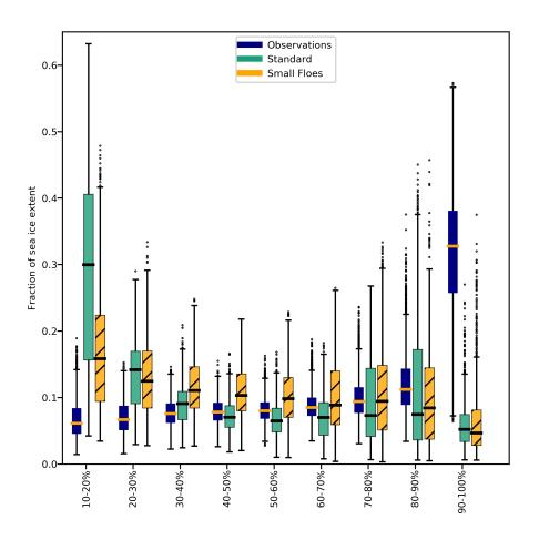
Figure 6. The fraction of sea ice extent in concentration bins for all days in each year from 2000 to 2014 in DJF from the three sets of observations, the standard NEMO-CICE ice-ocean model, and the NEMO-CICE ice-ocean model with small floe diameter L = 1 m. Boxplots as in Fig. 2. Hatching on the small floe simulation populations denotes that they are statistically different from the corresponding population from the standard model according to a Student's t-test (p < 5%)
