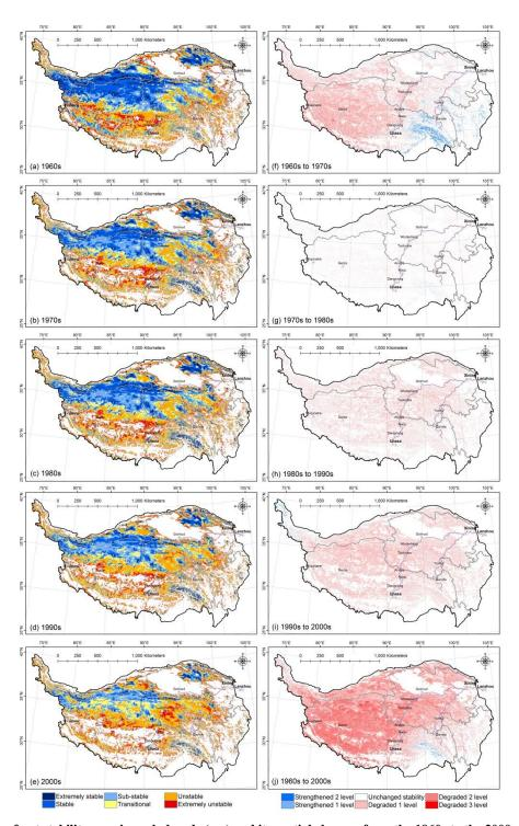
Figure 4. The permafrost stability map in each decade (a-e) and its spatial changes from the 1960s to the 2000s (f-j) over the QTP during the past 50 years.
