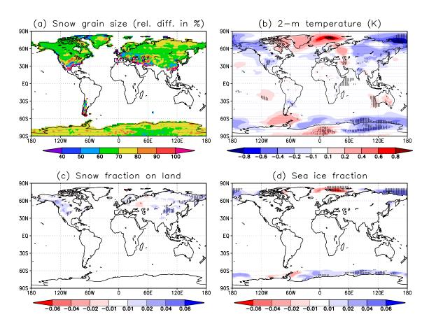
Figure 11. Annual-mean differences between the TUNED and SPH experiments: (a) the relative difference in the snow grain effective radius in the uppermost snow layer on land (in %), (b) the difference in 2-m air temperature (K), (c) the difference in snow fraction on land, and (d) the difference in sea ice fraction. In (b)–(d), differences significant at the 5% level are indicated with vertical hatching.
