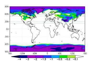
**Figure 2.** Annual-mean instantaneous radiative effect at the top of the model atmosphere  $(W m^{-2})$  due to changing the snow grain shape assumption from spheres to the OHC, evaluated through diagnostic radiation calculations in the SPH experiment.
