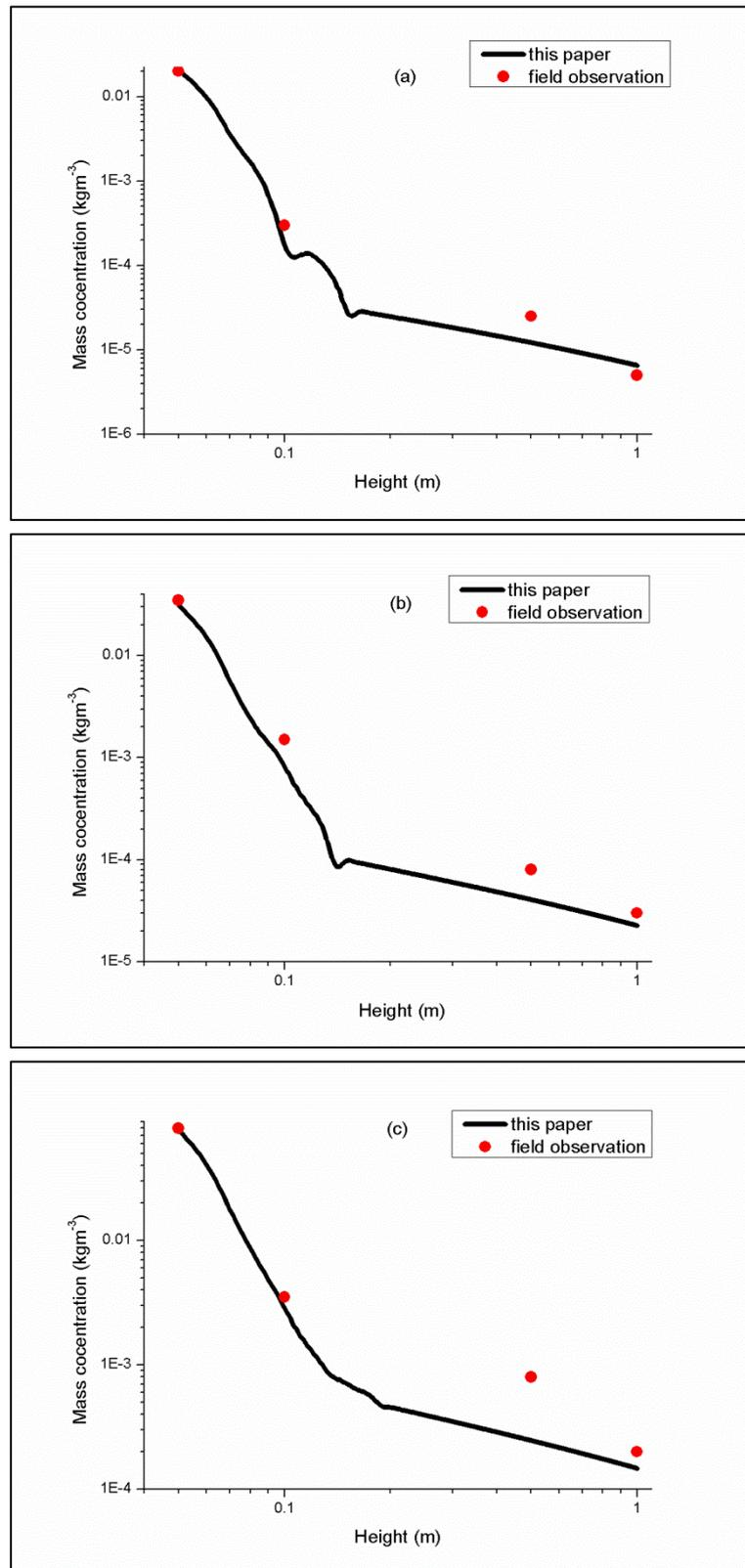
**Figure 2: Comparison of mass concentration for this paper and field observation (a:  $u_* = 0.35\text{ms}^{-1}; T = 268.65\text{K}$  ; b:  $u_* = 0.41\text{ms}^{-1}; T = 268.65\text{K}$  ; c:  $u_* = 0.54\text{ms}^{-1}; T = 268.65\text{K}$  ). The results of red dot are from near Saskatoon, Canada in 26 January 1987.**
