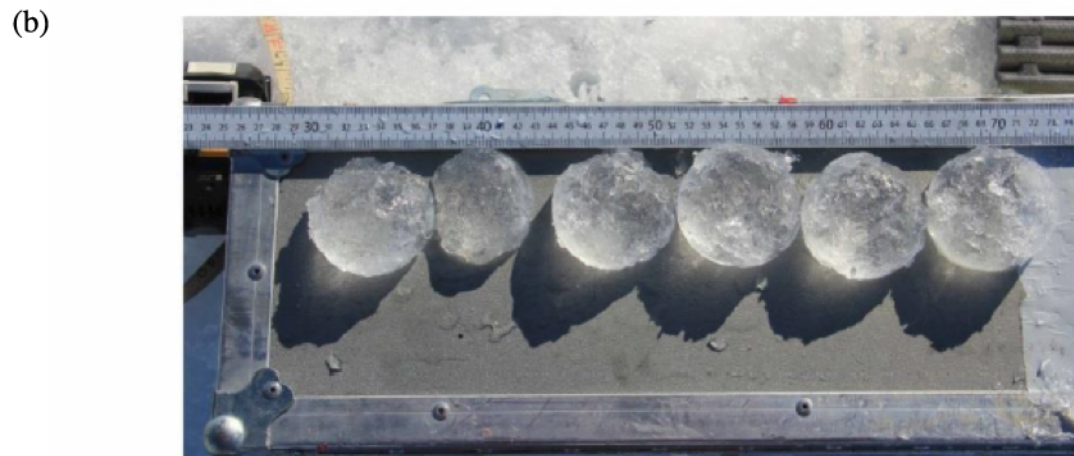
Fig. 5. (a) Typical near-surface shallow ice core (core #6) prior to in situ analysis of density and stratigraphy. Clear, solid ice lenses alternate with granular, fractured ice. Approximate locations of ice lenses noted with white arrows (not all lenses are clearly visible). (b) Ice lenses removed and confirmed after completed core analysis (core #1).
