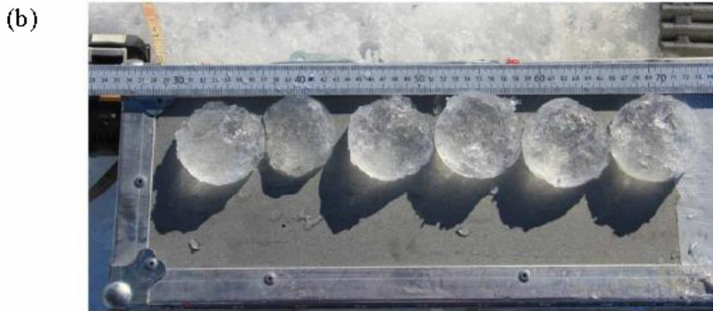
**Figure 4: (a) Typical near-surface shallow ice core (core #6) prior to in situ analysis of density and stratigraphy. Clear, solid ice lenses alternate with granular, fractured ice. (b) Ice lenses removed and confirmed after completed core analysis (core #1).**
