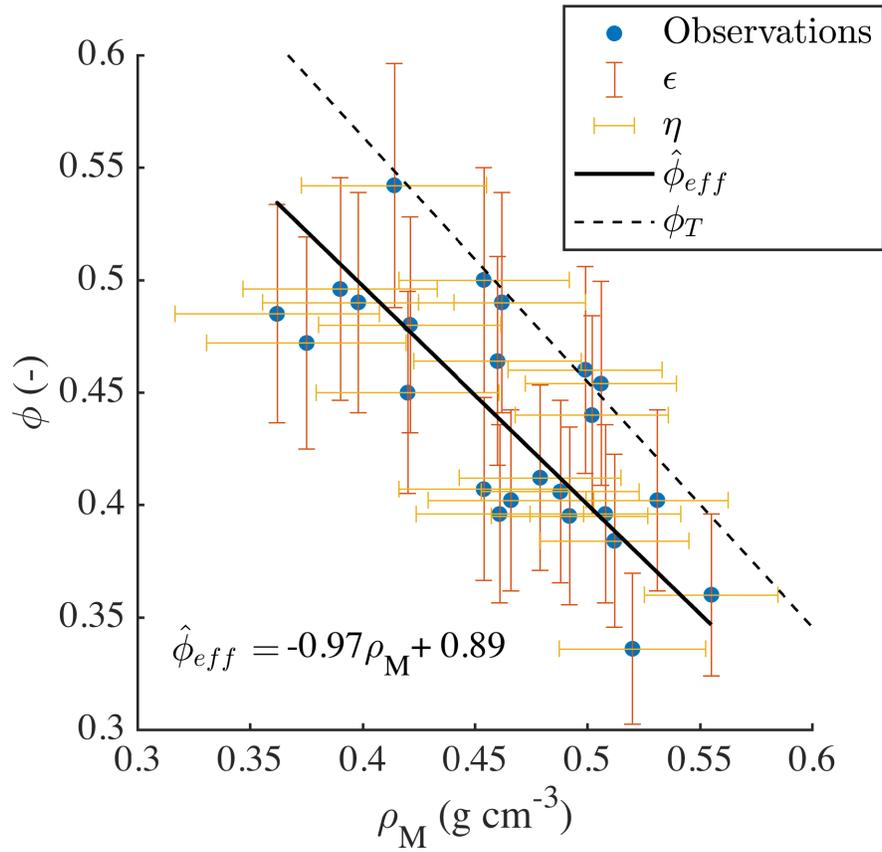
**Fig. 5:** Linear relationship ( $\hat{\phi}_{eff}$ , solid line) between measured ice density ( $\rho_M$ ) and effective porosity ( $\phi_{eff}$ ) and assumed  $\pm 10\%$  measurement error (whiskers). Dashed line is theoretical upper limit where effective porosity equals total porosity (i.e.  $\phi_T = \rho_M / \rho_T$ ).
