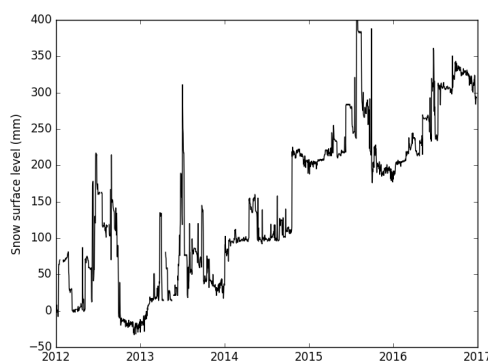
Figure 10. Snow surface level in mm above the reference level of the 1 st of January 2012 obtained from acoustic distance measurements. Presented daily mean values were calculated from measurements recorded every 30 minutes and corrected for air temperature.
