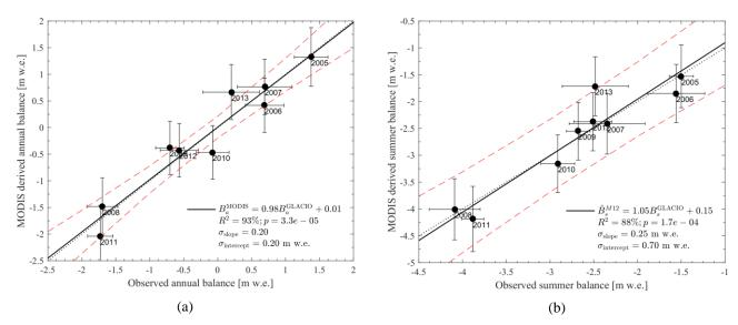
Figure 11. Relationship between MODIS-derived balance for (a) annual balance with Model M1 and (b) summer balance with Model M12. The dotted line is the 1:1 ratio. The dash line is the standard error prediction interval.
