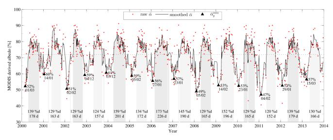
Figure 8. Time-series of MODIS-derived glacier-wide albedo  $\overline{\alpha}(t)$ . The shaded sections indicate the areas under which the signal was integrated to measure the cumulative winter albedo value  $A_y$ . The contrasting annual minimum albedo values  $\overline{\alpha}_y^{\min}$  are also evident.
