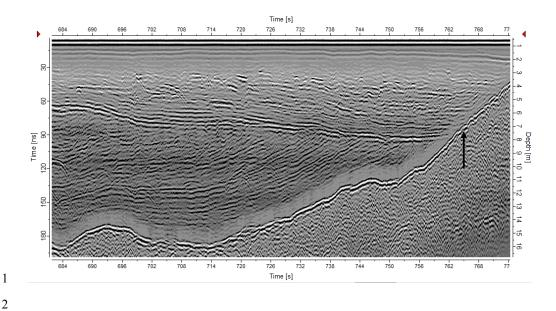
Figure 4. Example of 500 MHz Georadar profile. The position of the track shown in figure 3b. The arrow shows minimum front position in September 2014 (Ice velocity: 168 m  $\mu$ s-1, adjustment velocity: 300 m  $\mu$ s-1, automatic gain control, scale factor 5000).
