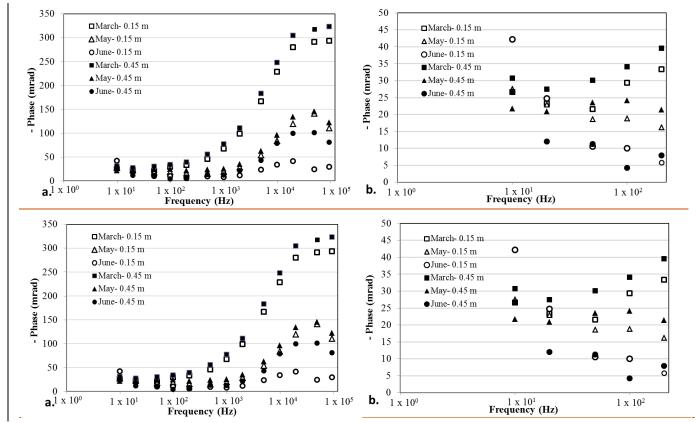
Figure 9: Phase of 2013 complex conductivity as a function of frequency (a) From 0 Hz to 95 kHz (b) From 0 to 200 Hz.
