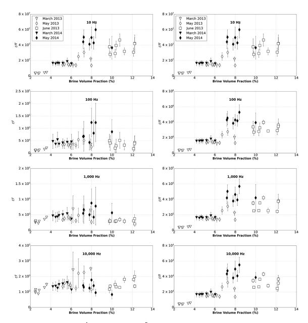
**Figure 8:** Variation of the real ( $\mathcal{E}'$ ) and imaginary ( $\underline{\mathcal{E}''}\underline{\mathcal{E}''}$ ) parts of the measured permittivity as a function of brine volume fraction. Squares – late March, diamonds – mid May, triangles – early June. Open symbols – 2013, filled symbols – 2014.
