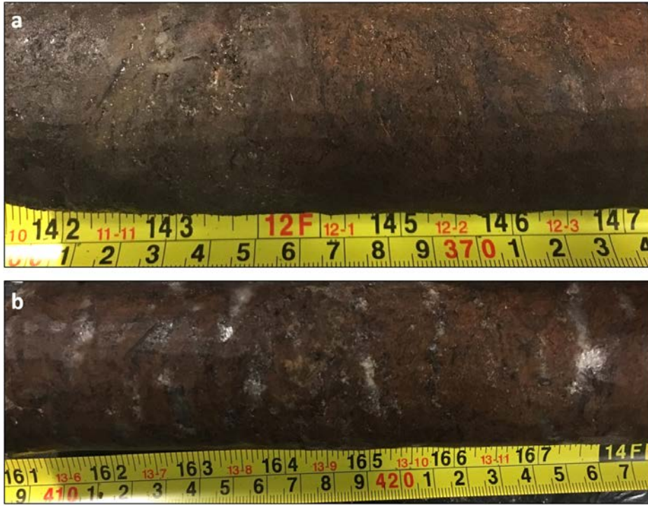
Figure 9: (a) Stratigraphic contact between the base of the frozen silt and peat layer occurring at 3.65 m and the underlying frozen peat. (b) Example of organic-matrix microlenticular to suspended cryostructures developed in the peat below the stratigraphic contact shown in (a).
