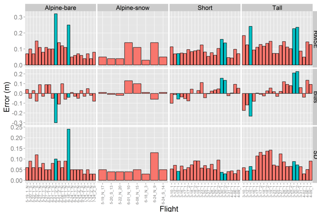
620 621 Figure 4: Root mean square error (RMSE, top row), Bias (middle row) and standard deviation (SD) of 622 DSMs with respect to surface over alpine-bare, alpine-snow, and short and tall stubble at prairie site, 623 respectively. Blue bars highlight problematic flights and are excluded from summarization in Table 1. X- 624 axis labels represent month-date-flight number of the day (to separate flights that occurred on the same 625 day). Alpine-bare accuracies are separated into north or south areas, reflected as _N or _S at the end. 626 The last number in the alpine-snow x-axis label is the number of observations used to assess accuracy as 627 they vary between 3 and 20.
