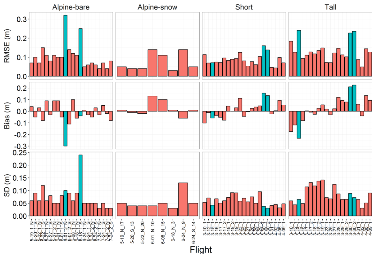
Figure 4: Root mean square error (RMSE, top row), Bias (middle row) and standard deviation (SD, bottom row) of DSMs with respect to surface over alpine-bare, alpine-snow, and short and tall stubble at prairie site, respectively. Blue bars highlight problematic flights and are excluded from summarization in Table 2. X-axis labels represent month-date-flight number of the day (to separate flights that occurred on the same day). Alpine-bare accuracies are separated into north or south areas, reflected with a _N or _S suffix. The last number in the alpine-snow x-axis label is the number of observations used to assess accuracy as the number of surface observations varied between 3 and 20.
