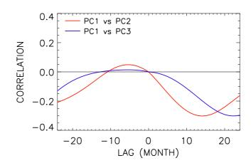
**Fig. 1.** Cross-correlation of the first PC time series against the second (red) and third (blue) PC time series for the lag range of (-24,24).
