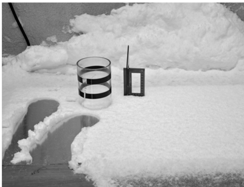
5 Figure 1: Accumulated snow on the thin metal plate on the table in the low-temperature room and the cylindrical sampler.
