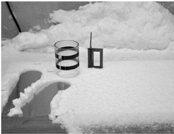
Figure 1: Photograph of the density observation set up in the low-temperature room, showing accumulated snow on a thin metal plate on the table, and the cylindrical sampler. As an indication of scale, the cylinder is 150 mm in height and 100 mm in diameter.
