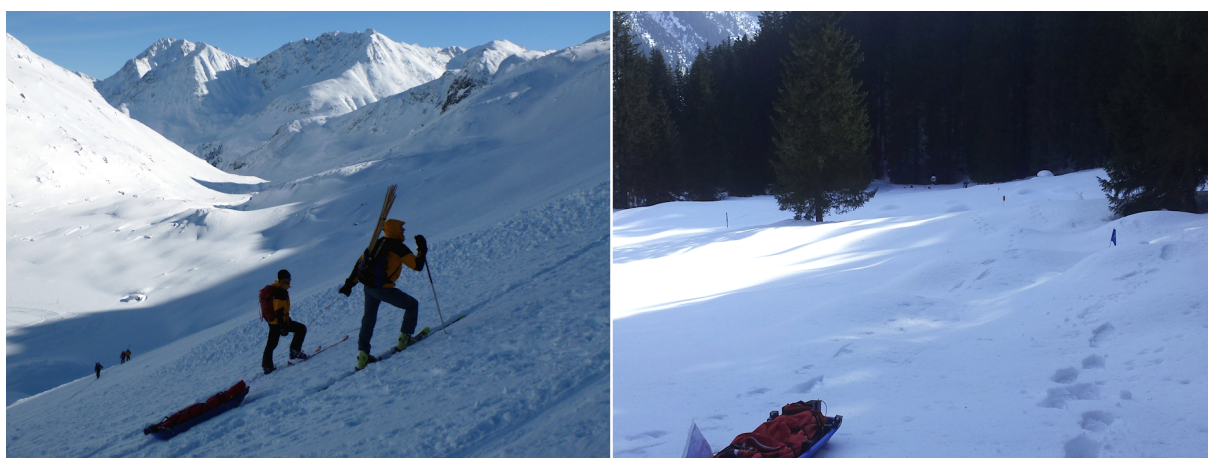
Figure 3. Fieldwork using GPR in steep alpine terrain (left) and (right) fieldwork at the third overpass of a transect in Monbiel valley. Flags mark points of manual measurements of snow depth and snow water equivalent for validation/calibration purposes, and serve as reference points for the synchronization of subsequent overpasses.
