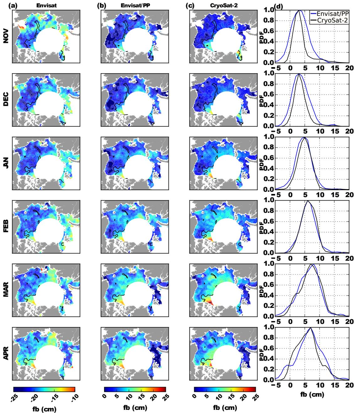
**Figure 6.** (a) Envisat, (b) Envisat/PP and (c) CryoSat-2 monthly freeboard maps shown for the November 2010 - April 2011 period. The dark lines represent the isoline fraction of MYI equal to 0.7. (d) Probability Distribution Function (PDF) of Envisat/PP (blue) and CryoSat-2 (black) radar freeboard.
