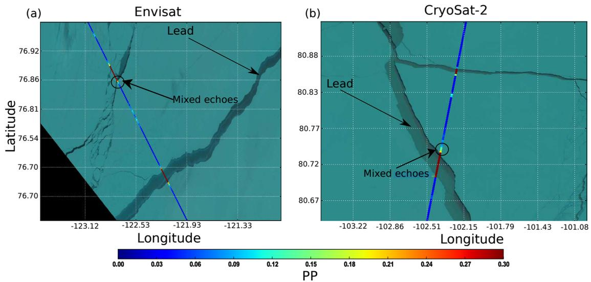
**Figure 1.** (a) PP spatial variability along Envisat track (16 April 2003) plotted over a Landsat-7 LandsatLook Image acquired on the same day and (b) PP spatial variability along CryoSat-2 track (01 May 2015) plotted over a Landsat-8 LandsatLook Image also acquired on the same day. For both figures, each dot represents a 20 Hz PP measurement.
