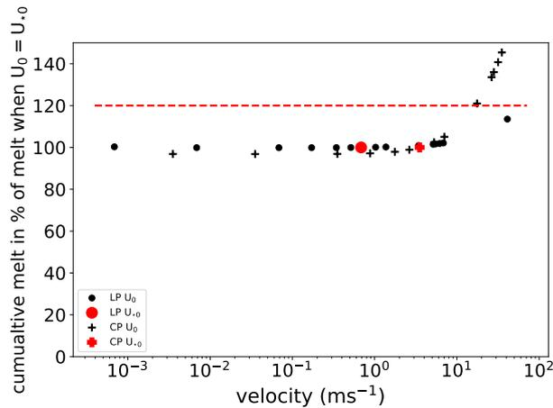
**Figure 3.** Sensitivity of cumulative melt rate to different initial velocities, for both plume models. Melt rate (black) is in percent of the cumulative melt achieved with initial balance velocity  $U_* U_{*0}$  (red). Red dashed line shows 120 % mark. Only very high initial velocities can **for the CP model** appreciably increase the cumulative melt rate **for the CP**.
