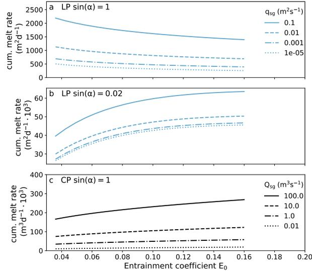
**Figure 6.** Cumulative melt rates of the different plume models as a function of the entrainment rate factor parameter  $E_0$  for four different discharge values. The cumulative melt rate is depicted for a) LP of a tidewater glacier ( $\sin(\alpha) = 1$ ), b) LP of a long floating tongue and c) CP of a tidewater glacier. For the LP model for  $\sin(\alpha) = 1$  a higher  $E_0$  leads to lower cumulative melting opposite to the other two cases.
