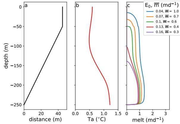
**Figure 13.** Kangerlussuup Sermia average undercut profile at the terminus (a) with the assumed temperature profile (b) give different melt rate profiles (c) simulated for different  $E_0$  and same  $Q_{sg} = 208 \text{ m}^3 \text{ s}^{-1}$ . All average melt rates are below the determined  $2 \text{ md}^{-1}$  by Fried et al. (2015).
