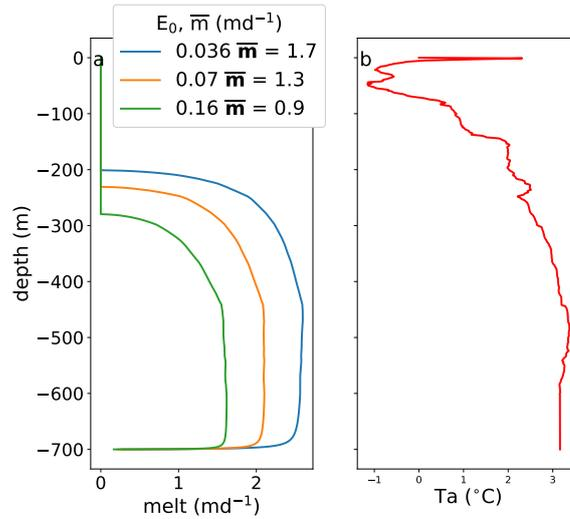
**Figure 14.** Three vertical melt rate profiles of the LP model (a) for three different entrainment coefficients  $E_0$  for Helheim glacier. With and a discharge of  $2.69 \cdot 10^{-2} \text{ m}^2 \text{ s}^{-1}$  and  $E_0 = 0.036$  we obtain an average melt rate of  $\bar{m} = 1.6 \text{ ma}^{-1}$  very  $\bar{m} = 1.7 \text{ ma}^{-1}$  close to Sutherland et. al Sutherland and Straneo (2012) ( $1.7-1.8 \text{ md}^{-1}$ ).
