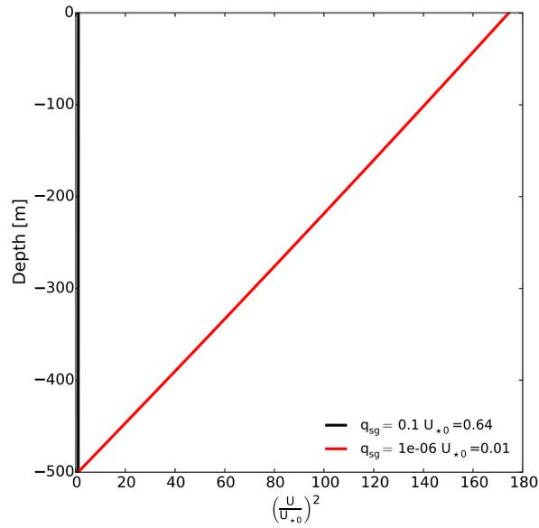
**Figure A2.** Evolution of  $U$  for an initial velocity of  $U_{*}$ . The plume with a small discharge ( $q_{sg} = 10^{-6} \frac{m^2}{s}$ ) will accelerate strongly (red line,  $U_{*} = 0.14 \frac{m}{s}$ ) while the plume velocity with larger discharge remains almost constant (black line,  $q_{sg} = 0.1 \frac{m^2}{s}$ ,  $U_{*} = 0.63 \frac{m}{s}$ ).
