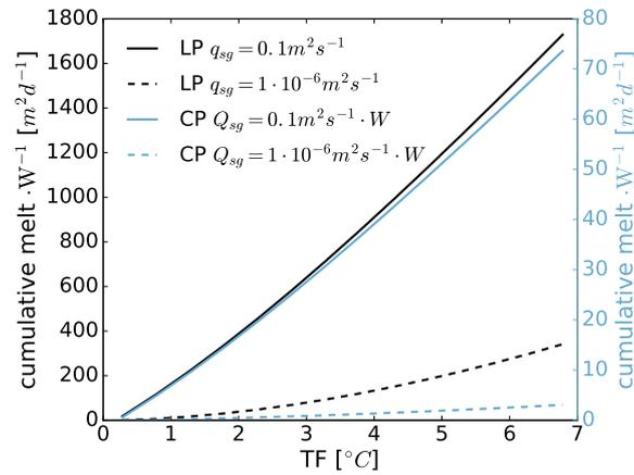
**Figure 8.** Cumulative melt rate per glacier width  $W$  for the LP model (black) and CP (blue) model as a function of the thermal forcing ( $TF = T_a - T_{af}$ )  $\Delta T_g = T_a - T_{gf}$  for high (solid lines) and low (dashed lines) discharge values. The experiment is for a well-mixed, 500m deep and 5km wide tidewater glacier ( $\sin(\alpha) = 1$ ), with  $S_a = 34$  psu and  $E_0 = 0.1$ .
