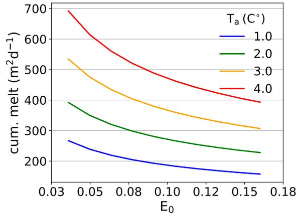
**Figure 7.** cumulative Cumulative melt rate in dependence of the LP as a function of entrainment parameter  $E_0$  for  $q_{sg} = 10^{-3} \text{ m}^2 \text{ s}^{-1}$  in four different well mixed ambient Temperatures ( $T_a$ ), in a tidewater glacier.
