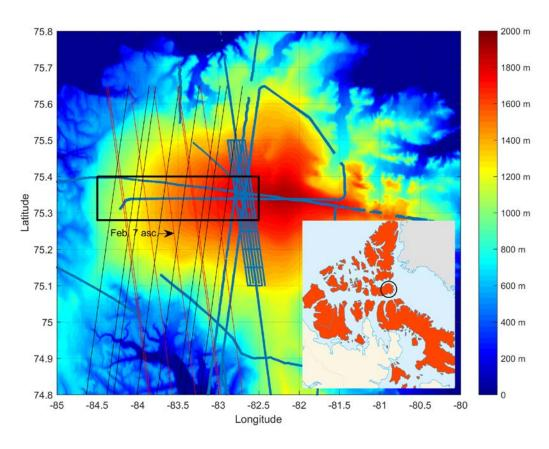
5 Figure 1: Location of the test area on the western slopes of the Devon Ice Cap (black rectangle). The sub-satellite positions of the spring 2011 ascending and descending passes crossing the test area are shown by the red and black lines respectively. The positions of the reference surface height data are shown in blue. The insert shows the position of Devon Ice Cap (circled) in the Canadian Arctic Archipelago.
