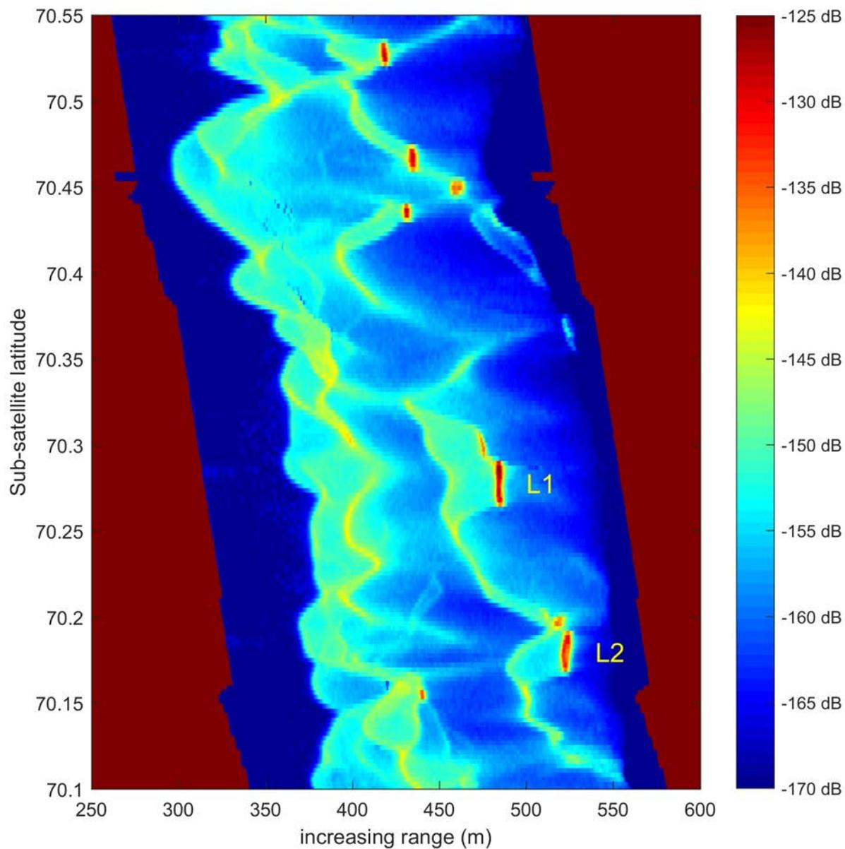
5 **Figure 13. Illustration of part of the waveform power from an ascending pass over west Greenland on 7 August 2011 (Fig. 14). The bright returns labelled as L1 and L2 are at elevations ~ 1609 m and 1573 m, respectively, and represent topographic lows where water could collect.**
