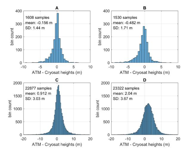
Figure 9. Comparisons of the west Greenland ATM – CryoSat height difference histograms for the solution using the pre-launch baseline coupled with an additional roll offset (A; POCA, C; swath mode solutions). Boxes B and D use the Galin et al. (2013) calibration for the POCA and swath solutions respectively.
