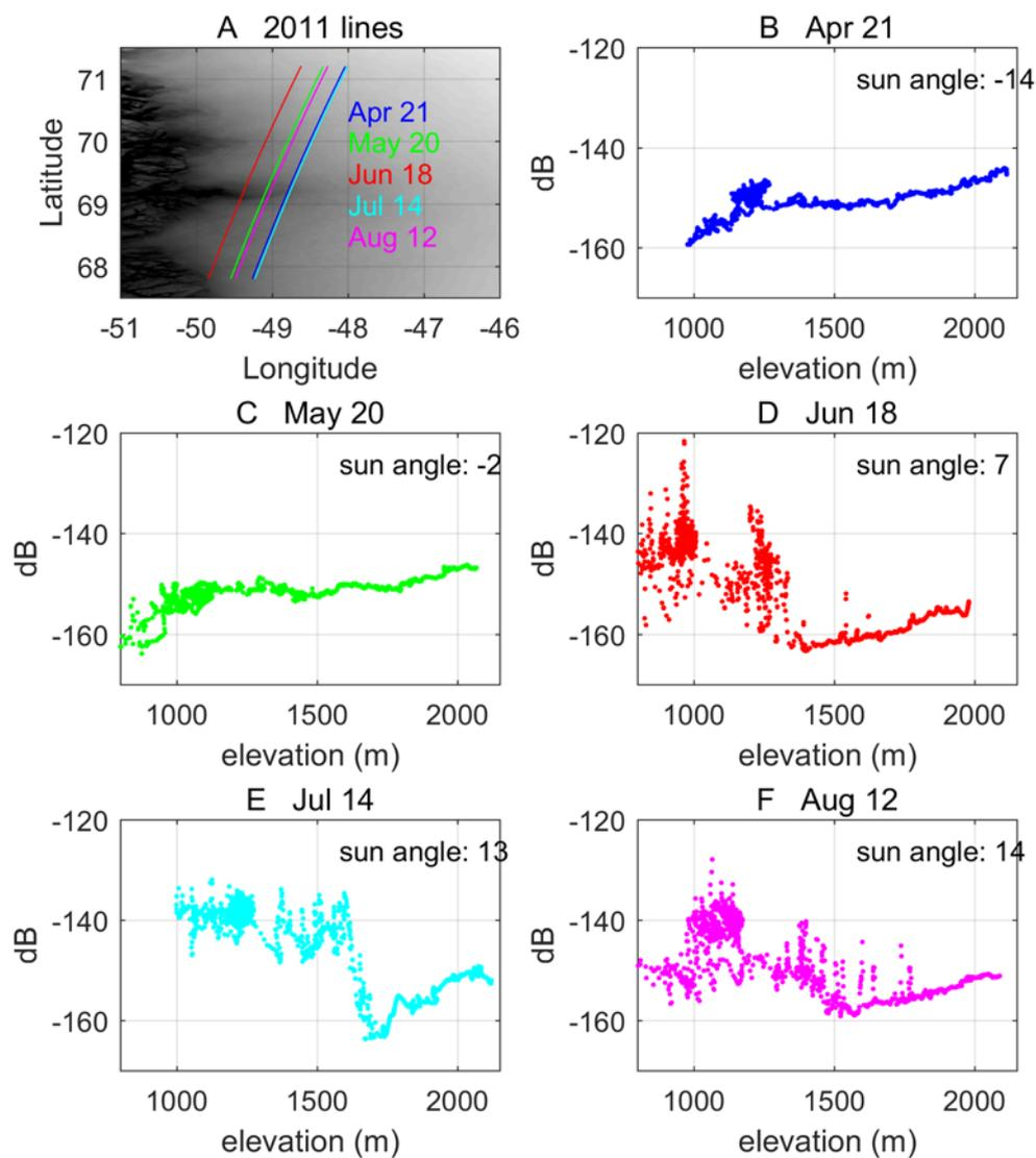
5 **Figure 12.** Plots of the average waveform power for the five 2011 descending passes shown in (A). The five plots are from descending passes on (B) April 21, (C) May 20, (D) June 18, (E) July 14 and (F) Aug. 12, and illustrate average waveform power as a function of elevation.
