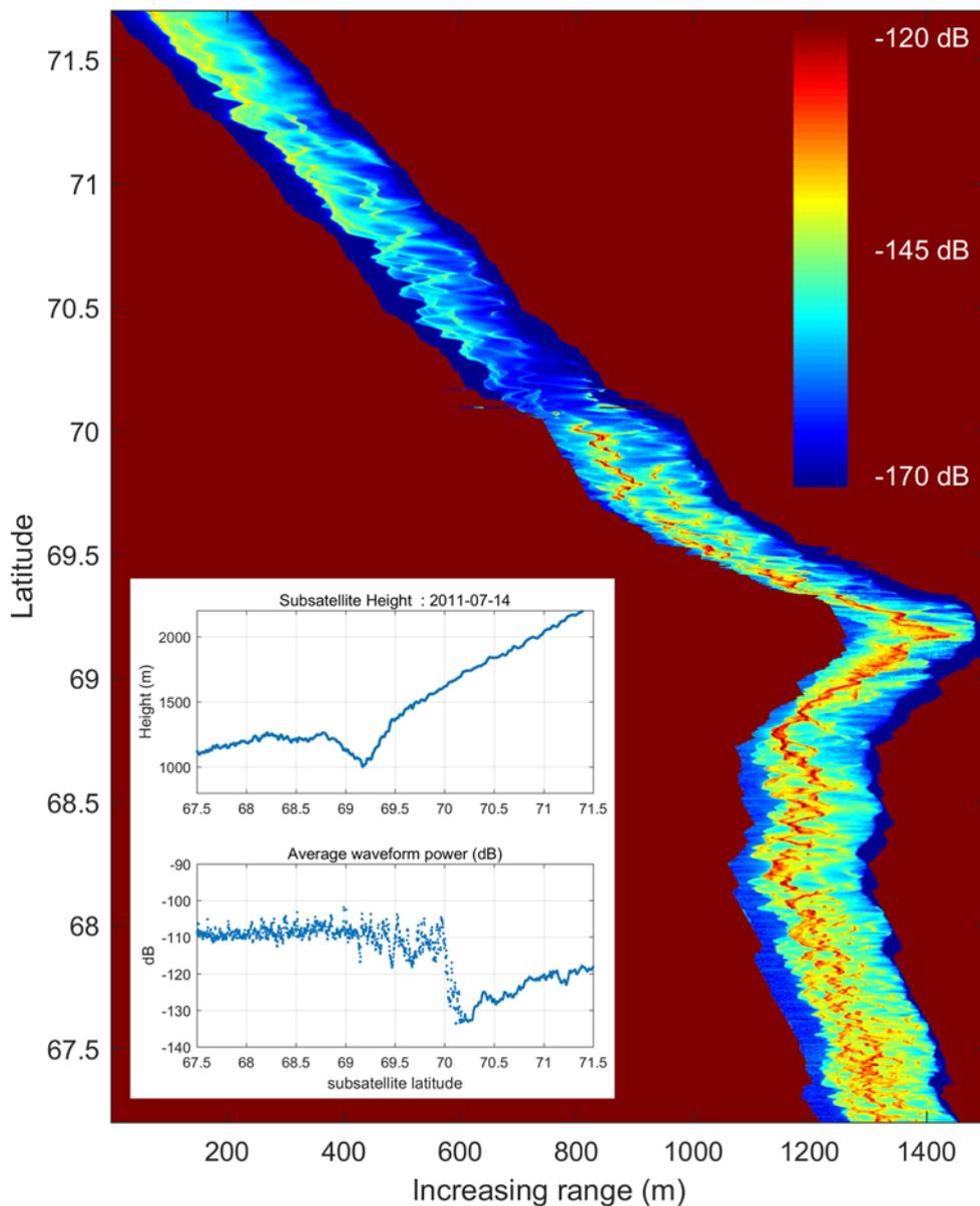
5 **Figure 11.** The background image illustrates the swath waveform power in colour with a dB scale for the July 14 2011 descending pass over the west Greenland test area (Fig. 12A). The waveforms making up this pseudo-image have been shifted in the x direction to account for the changing delay time to the first sample and the varying satellite height above the WGS84 ellipsoid. The insert shows the sub-satellite terrain elevation and the waveform average power both plotted against latitude.
