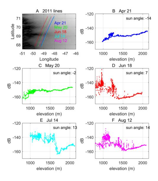
Figure 12. Plots of the average waveform power for the five 2011 descending passes shown in (A). The five plots are from descending passes on (B) April 21, (C) May 20, (D) June 18, (E) July 14 and (F) Aug. 12, and illustrate average waveform power as a function of elevation.
