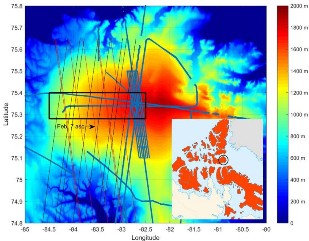
5 **Figure 1: Location of the test area on the western slopes of the Devon Ice Cap (black rectangle). The sub-satellite positions of the spring 2011 ascending and descending passes crossing the test area are shown by the red and black lines respectively. The positions of the reference surface height data are shown in blue. The insert shows the position of Devon Ice Cap (circled) in the Canadian Arctic Archipelago.**
