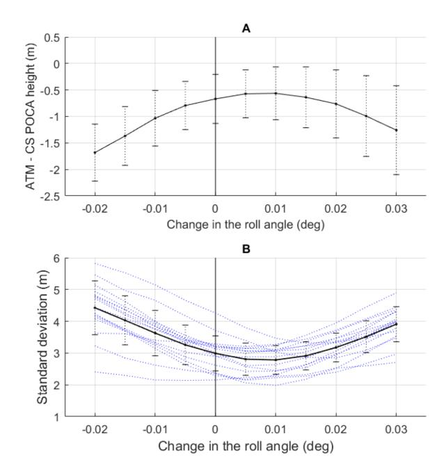
Figure 10. Illustration of the average of the ATM – CryoSat height differences for: (A) 16 passes plotted against the additional roll angle bias used in the processing (top). The error bars are  $\pm$  1 standard deviation about the mean. (B) Variation in the standard deviation (SD) of the ATM – CryoSat height difference for the individual passes (blue dotted lines) and the average over all the passes (solid black line).
