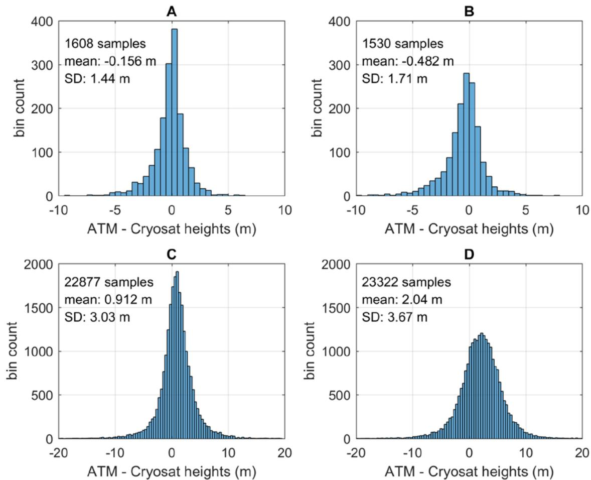
5 **Figure 9.** Comparisons of the west Greenland ATM – CryoSat height difference histograms for the solution using the pre-launch baseline coupled with an additional roll offset (A; POCA, C; swath mode solutions). Boxes B and D use the Galin et al. (2013) calibration for the POCA and swath solutions respectively.
