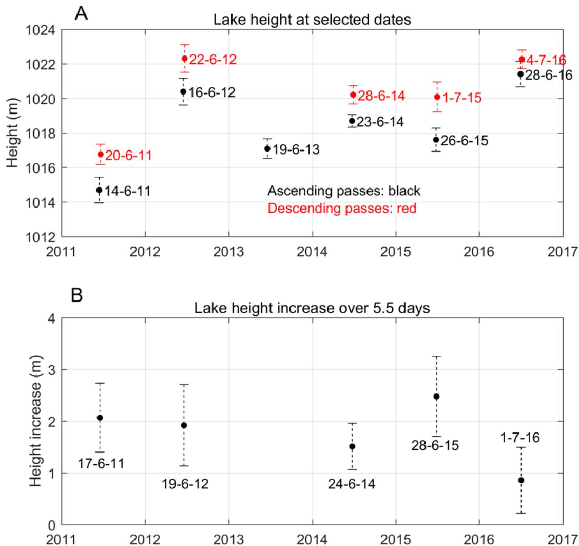
**Figure 18. (A) Surface height of the lake in Fig. 17 at the times of the overpasses: (B) Height increase during the 5.5 days between the ascending and descending passes. The dates listed in the lower plot are at the middle of the 5.5-day period between the ascending and descending passes.**
