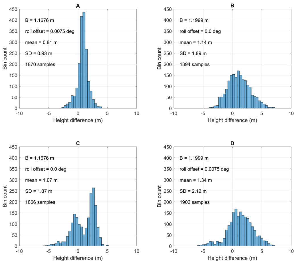
5 **Figure 5: Histograms of the reference minus CryoSat swath heights for Devon Ice Cap: (A) pre-launch baseline and a roll angle offset of 0.0075°; (B) modified baseline with zero roll offset; (C) pre-launch baseline with zero roll offset; and (D) modified baseline with a roll offset of 0.0075°.**
