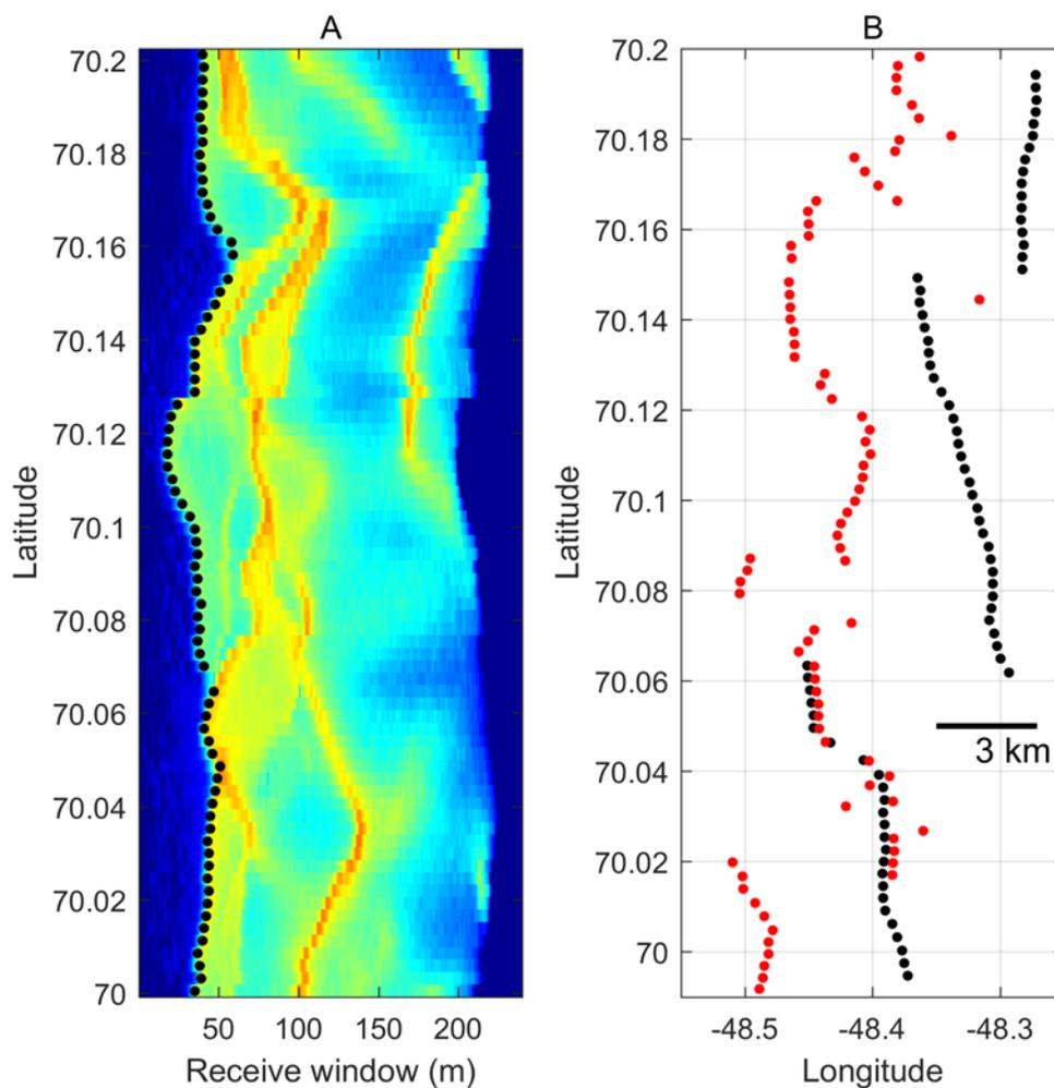
5 **Figure 7. (A) Waveform power without any x axis shifts using the same dB colour scale as in Fig. 6B. The detected POCA positions are shown in (A) for each waveform with black dots, and they clearly correspond to the leading edge of the waveforms. (B) Geographic positions of the geocoded footprints (black dots) are compared to the positions of the ESA L2 solutions (red dots).**
