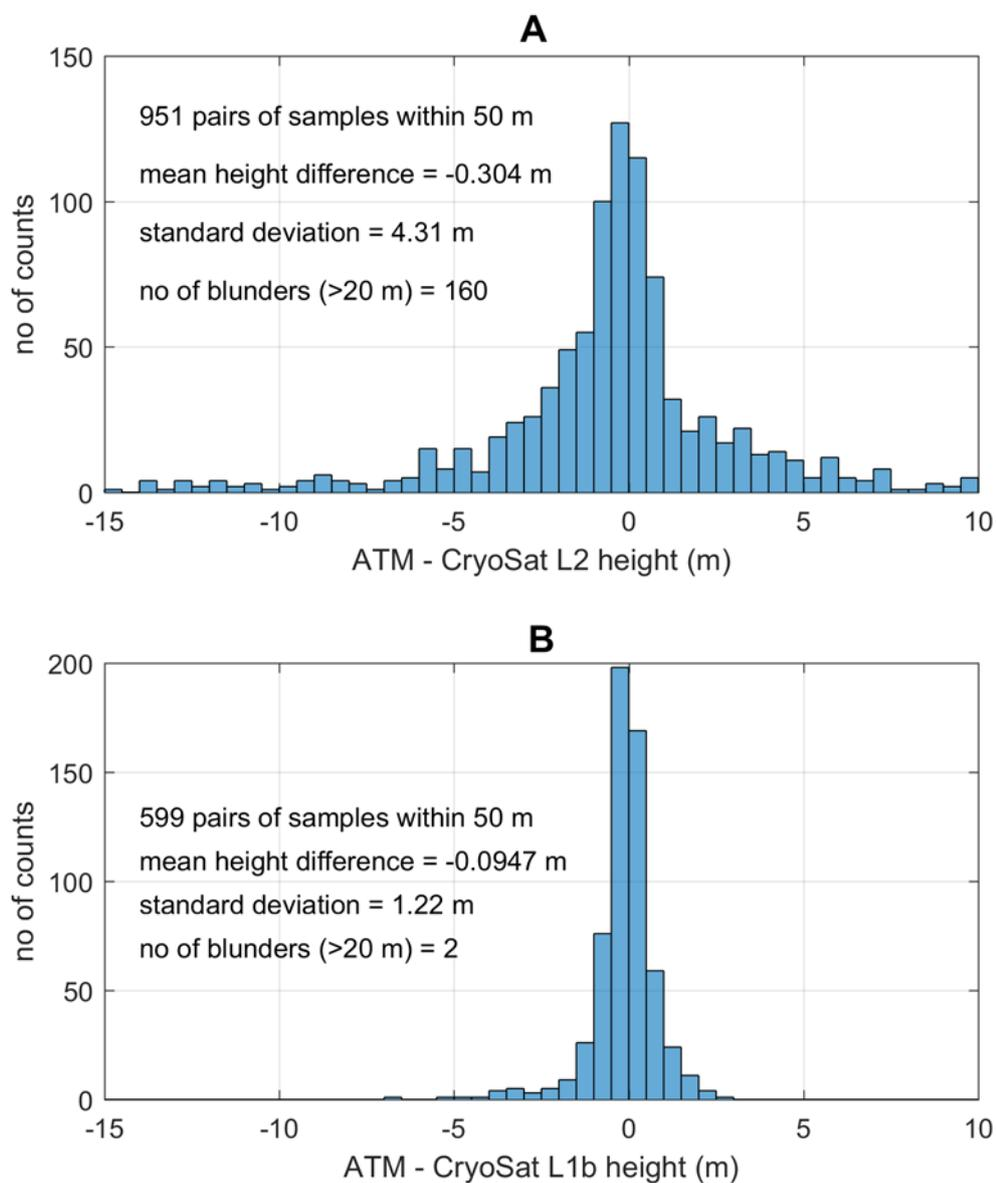
**Figure 8. Comparisons of the ATM - CryoSat POCA height difference histograms for the west Greenland test site. (A) the ESA L2 solution: (B) Results from the current maximum slope leading edge retracker.**
