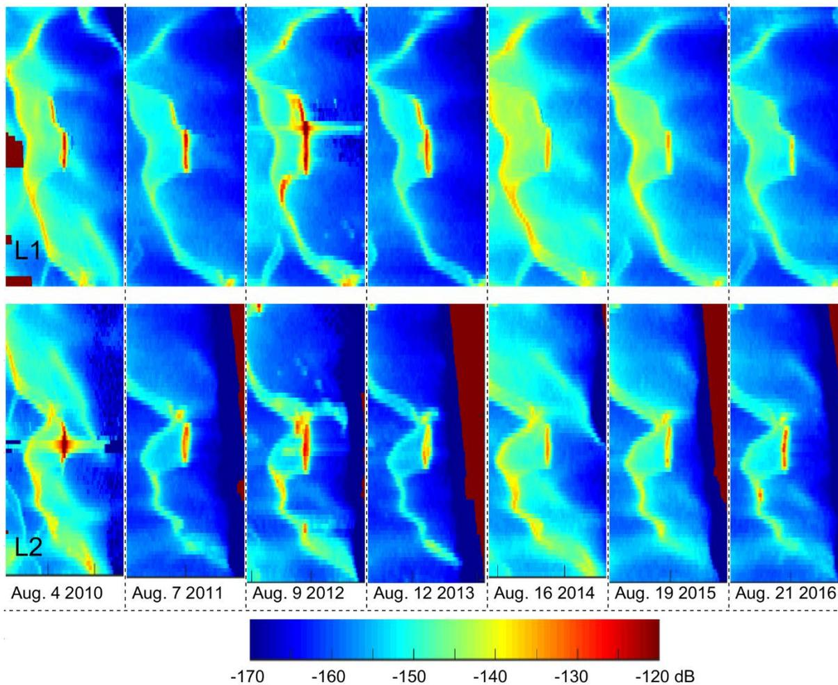
5 **Figure 15.** ‘Images’ of part of the CryoSat waveforms for the areas including ‘L1’ (top) and ‘L2’ (bottom) in west Greenland for the August dates in each year from 2010 to 2016.
